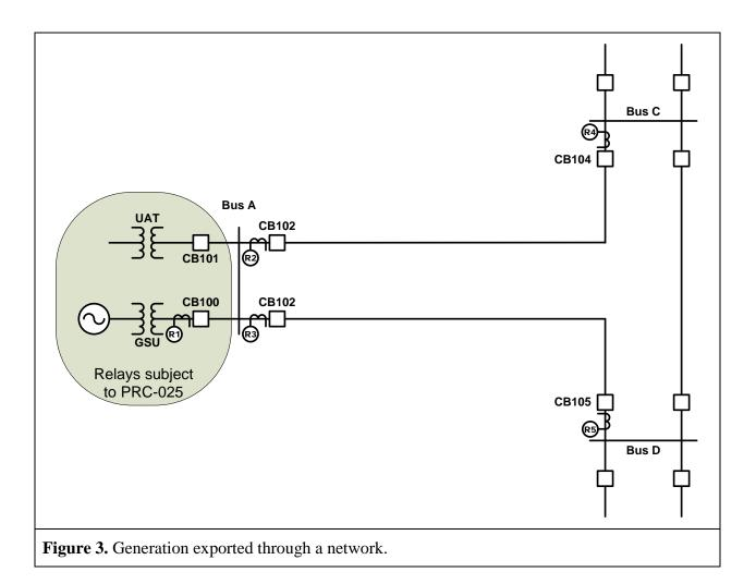
Elements utilized in the aggregation of dispersed power producing resources (in some cases referred to as a "collector system") consist of the Elements between individual generating units and the common point of interconnection to the Transmission system.
