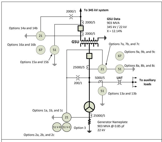
Figure 4. Relay Connection for corresponding synchronous options.
