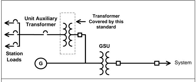
**Figure-7** – Typical auxiliary power system for generation units or plants.
