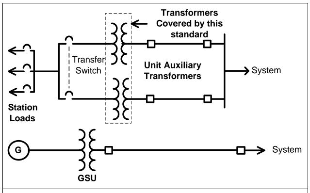
**Figure-6** – Auxiliary Power System (independent from generator).
