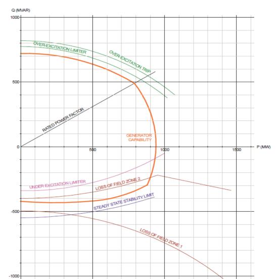
Section G Attachment 1 – Example of Capabilities, Limiters and Protection on a P-Q Diagram at nominal voltage and frequency
