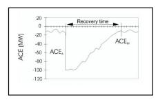
$$R_i = \frac{MW_{Loss} - \max(0, ACE_A - ACE_M)}{MW_{Loss}} * 100\%$$
