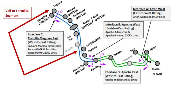
The following diagram reflects the rating interfaces for the proposed project:
