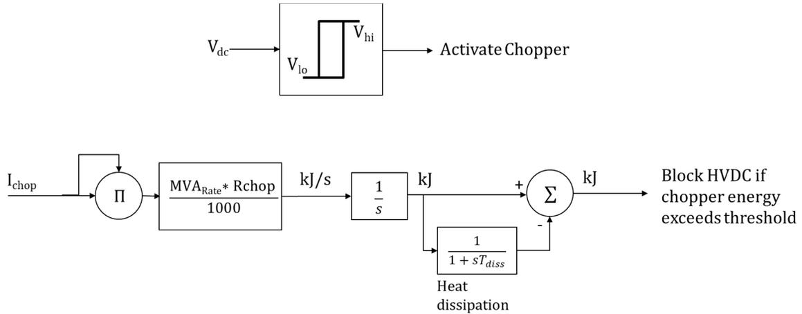
**Figure 8: Dc chopper energy dissipation-based protection.**
