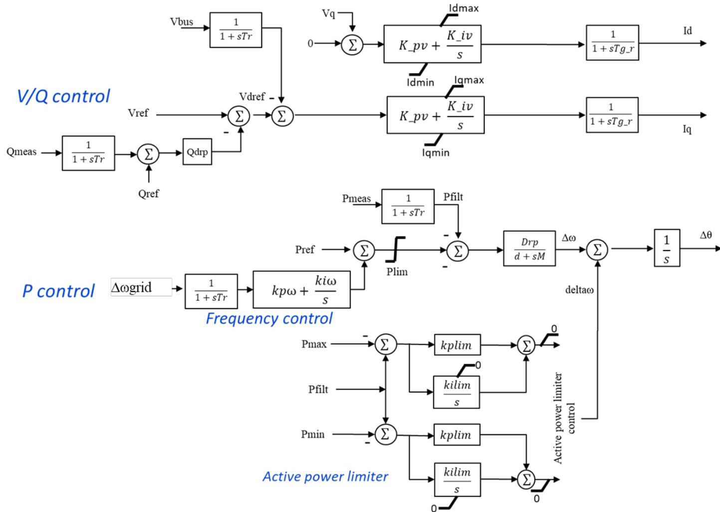
Figure 2 Grid forming control for the proposed VHVDC3 model.
