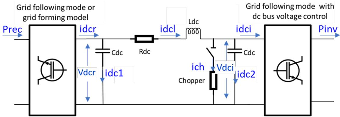
Figure 1 Dc line model for the proposed VHVDC3 model.
