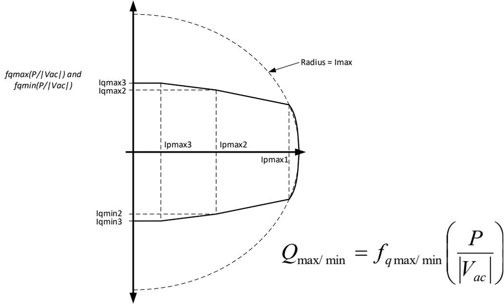
**Figure 7: Definition of the reactive power capability of both converters (D-curve) as a function of dc power transferred and ac voltage.**
