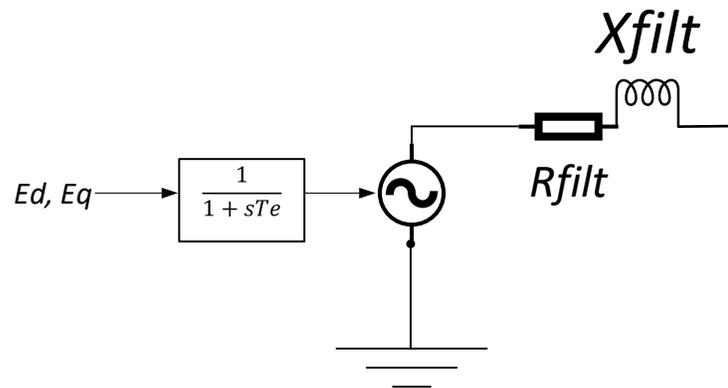
Figure 5 Network interface for the VSC HVdc model
