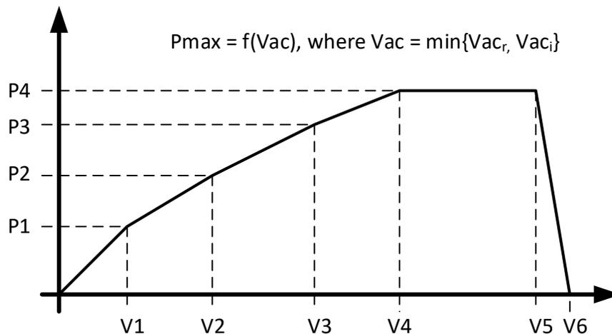
Figure 6 Power versus Voltage look-up table/curve for defining the maximum dc power reference as a function of ac voltage.
