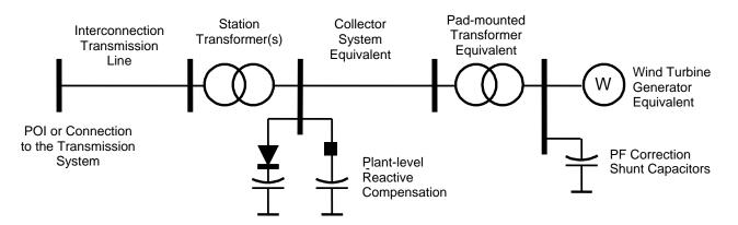
Figure 3: Single-Machine Equivalent Power Flow Representation
