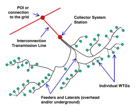
Figure 1. Wind Power Plant Topology
