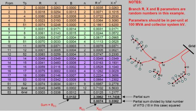
Figure 4 – Computation of Collector System Equivalent Parameters
