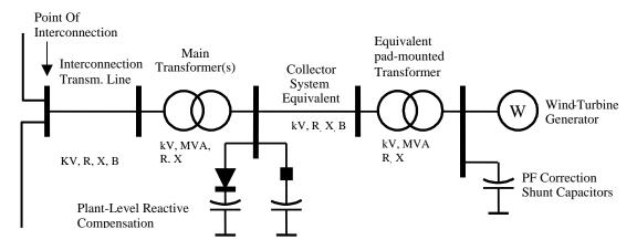
Figure A-1. Single-machine representation one-line diagram
