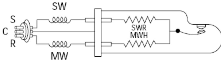
Figure 3. Thermal Overload Protection Switch
