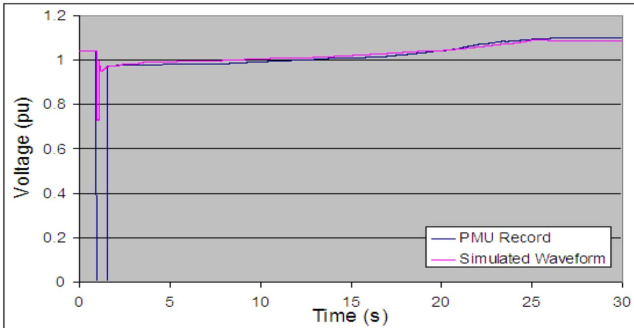
Figure 83. PSLF Simulation and PMU Comparison at 500 kV
