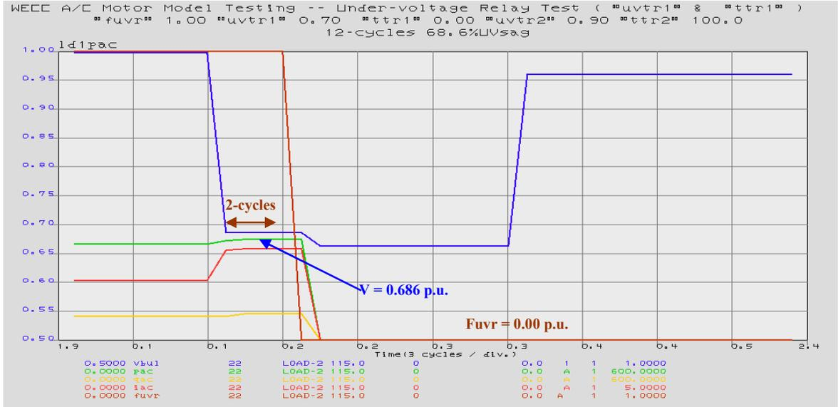
Figure 52. First UV Relay Tripping Parameters Test (uvtr1=0.70 & ttr1=0.00)
