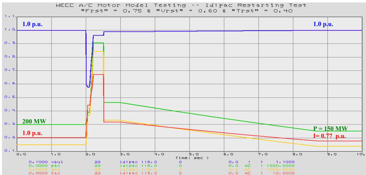
Figure 40. Restarting Fraction Test ( $Frst = 75\%$ )
