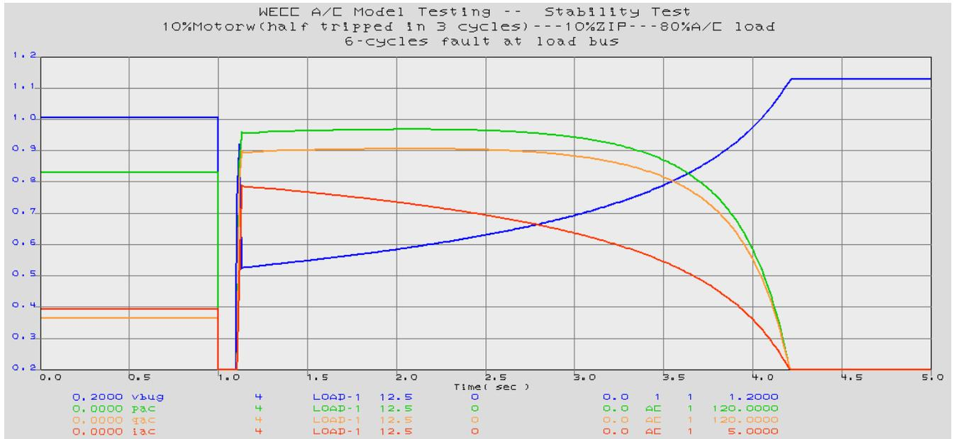
Figure 80. 6-Cycles Fault in the Load Bus
