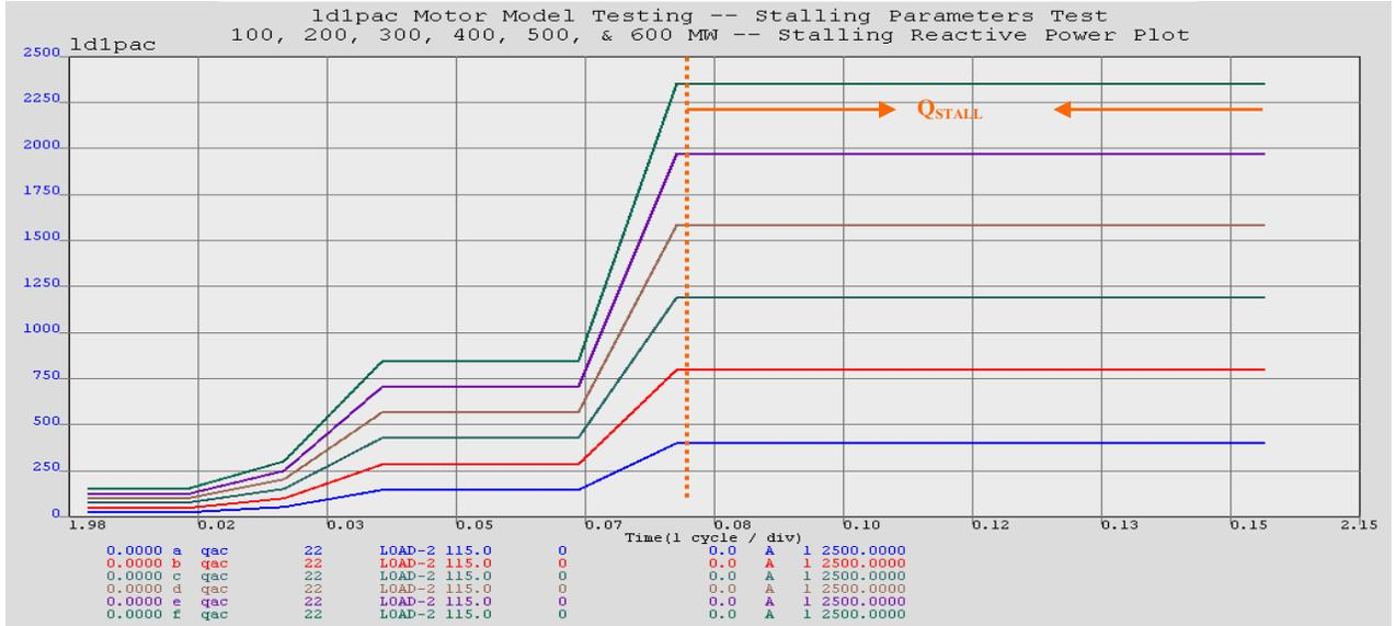
**Figure 78.** *Ldlpac* Model Parameters Test (Stall Reactive Power Plot)
