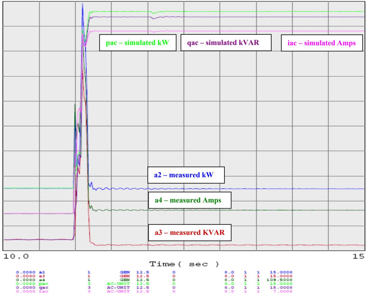
Figure 74. Voltage Sag: from 100% to 60% for 6 cycles with recovery to 90%
