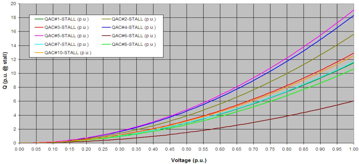
Appendix 2 -- Figure 3. Stall Reactive Power vs. Stall Voltage
