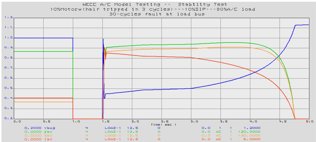
Figure 81. 30-Cycles Fault in the Load Bus
