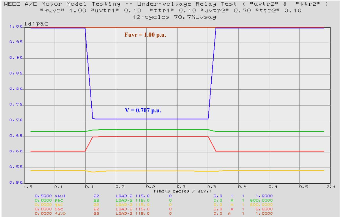
Figure 59. Second UV Relay Tripping Parameters Test ( $uvtr2=0.70$  &  $ttr2=0.10$ )
