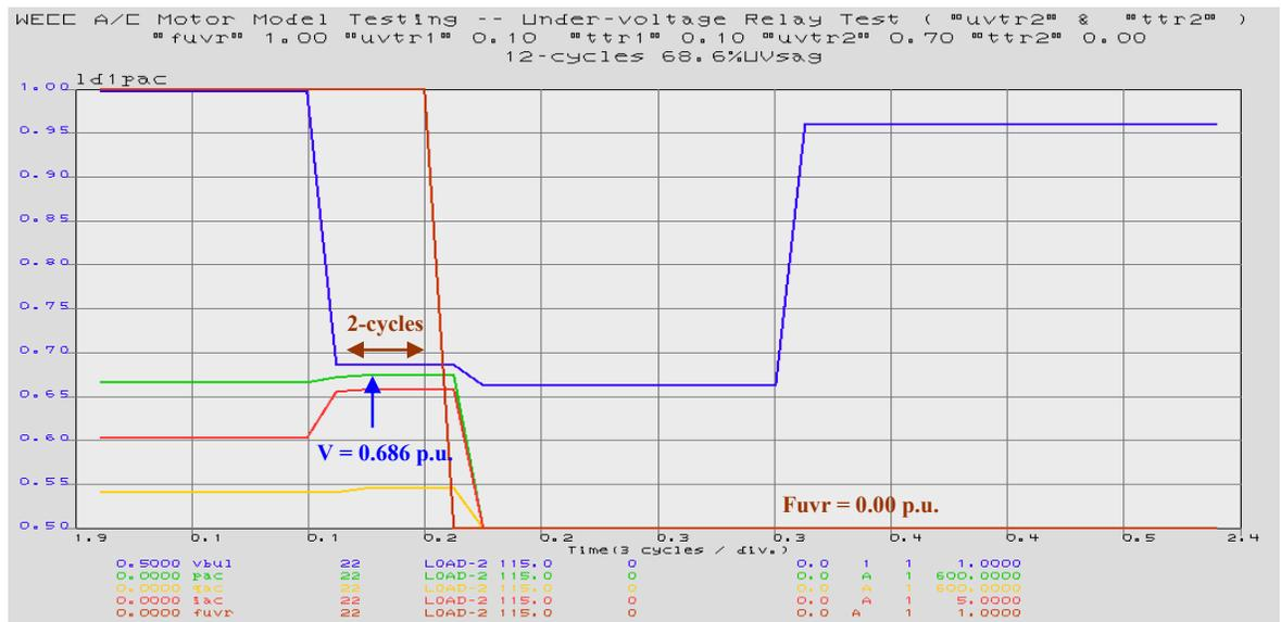
Figure 56. Second UV Relay Tripping Parameters Test (*uvtr2*=70% & *ttr2*=0.00)
