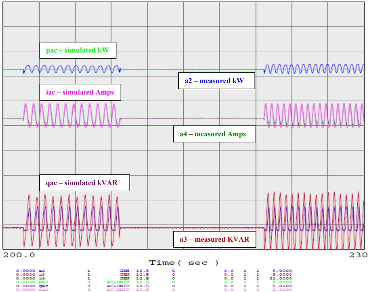
Figure 66. Voltage Oscillation at 1.0 Hz
