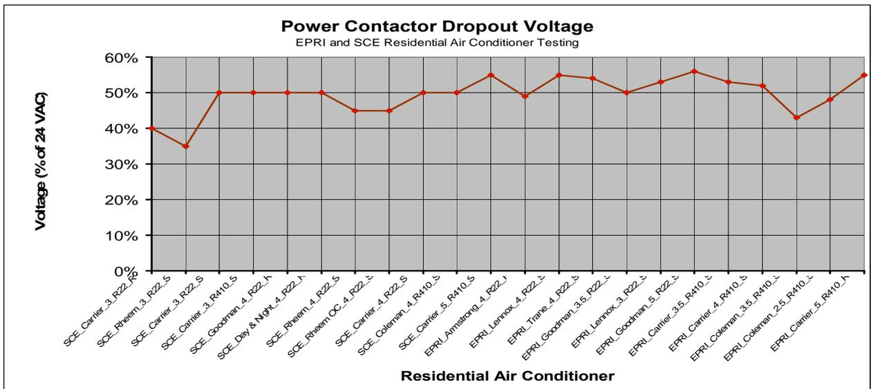
Figure 33. Power Contactor Dropout Voltages
