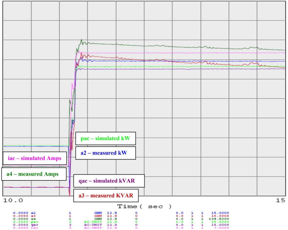
Figure 73. Voltage Sag: from 100% to 60% for 6 cycles with recovery to 80%
