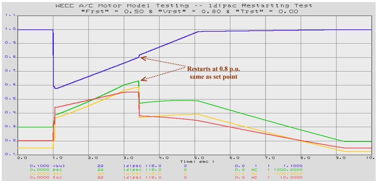
Figure 43. Restarting Voltage Test ( $V_{rst} = 80\%$ )
