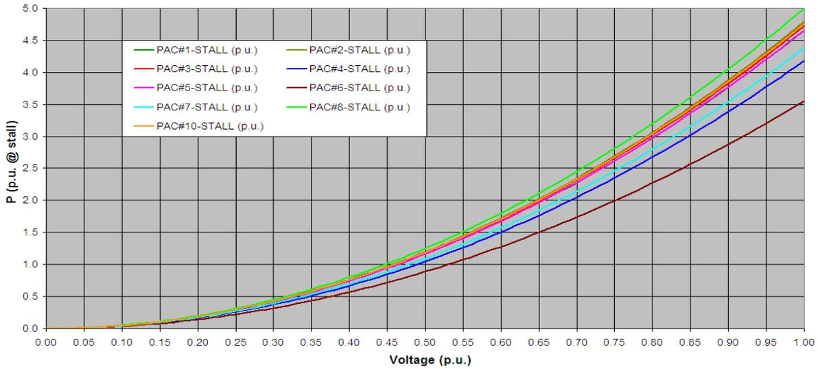
Appendix 2 -- Figure 2. Stall Real Power vs. Stall Voltage
