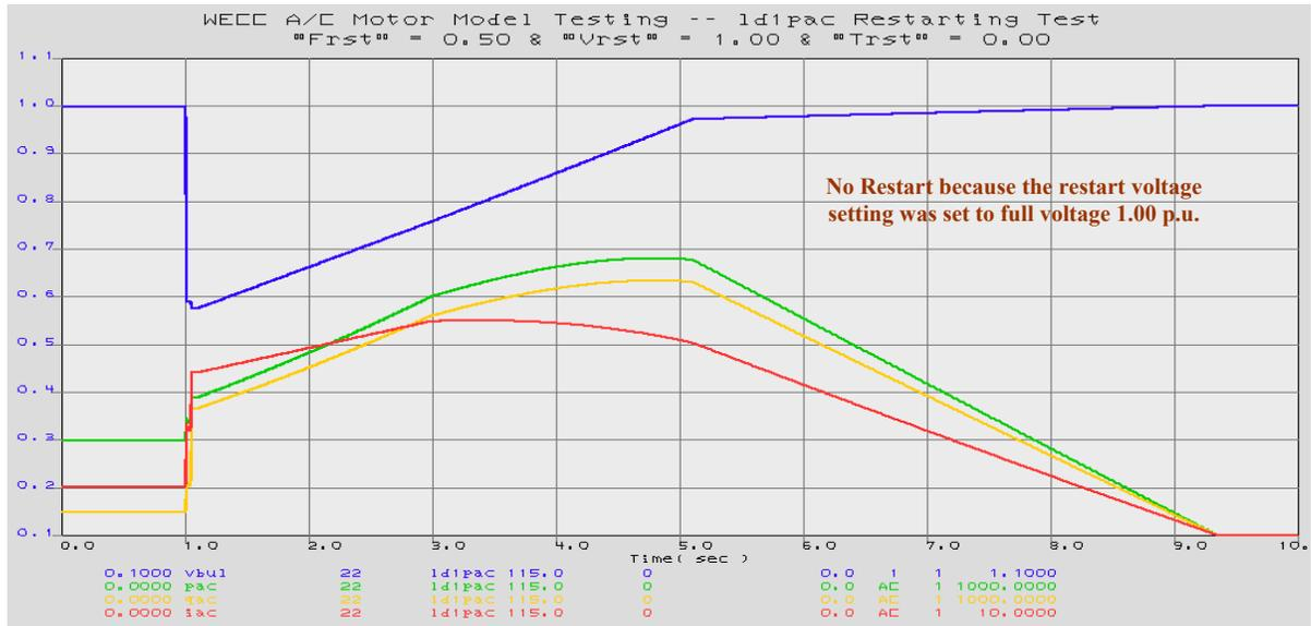
Figure 41. Restarting Voltage Test (Vrst = 100%)
