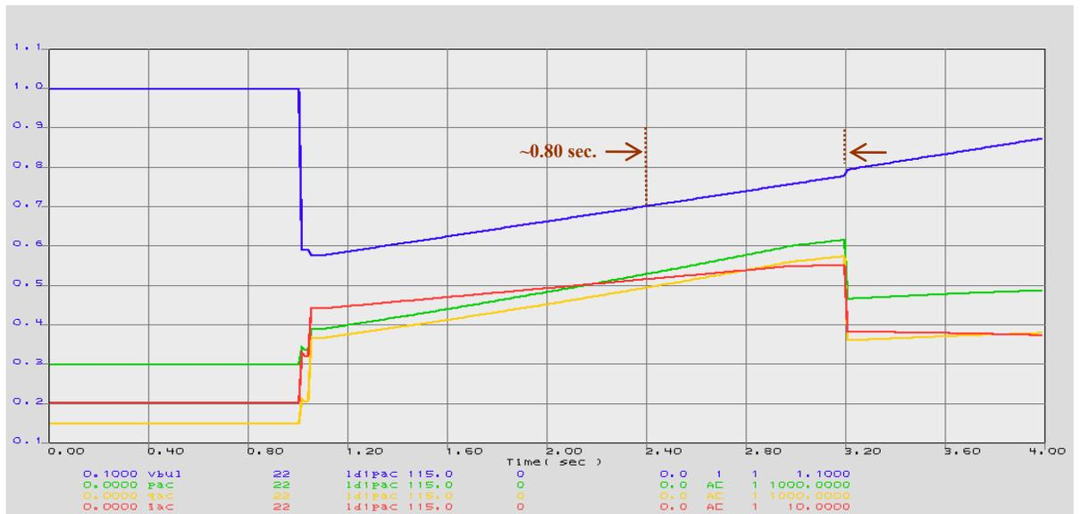
Figure 48. Restarting Delay Test ( $Trst = 0.80$ )
