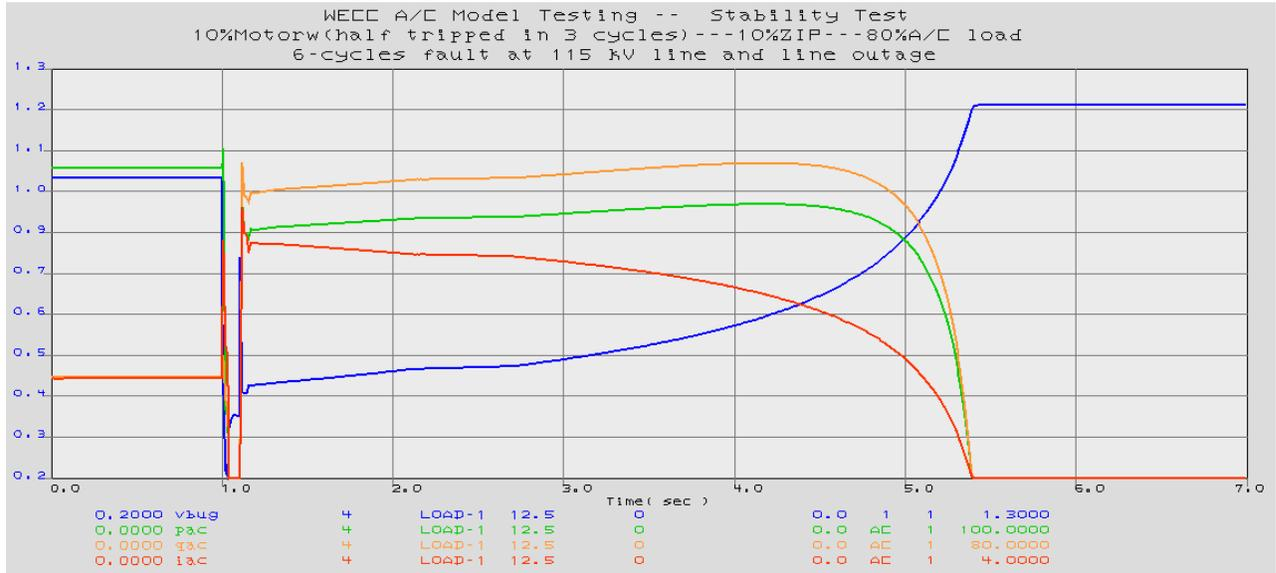
Figure 82. 6-Cycles Fault at Line and Line Clearance
