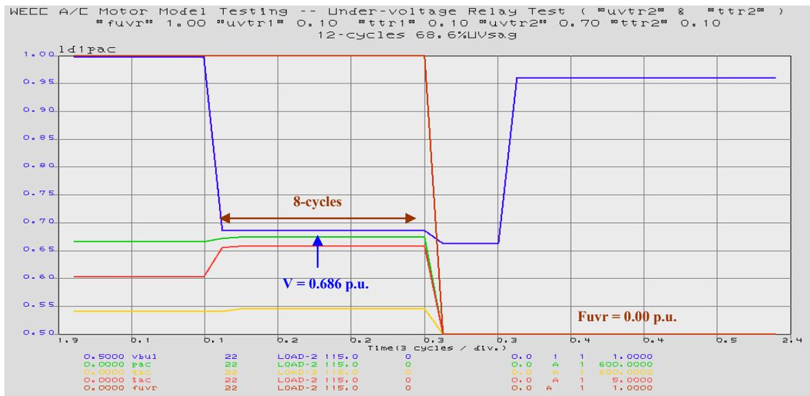
Figure 58. Second UV Relay Tripping Parameters Test ( $uvtr2=0.70$  &  $ttr2=0.01$ )
