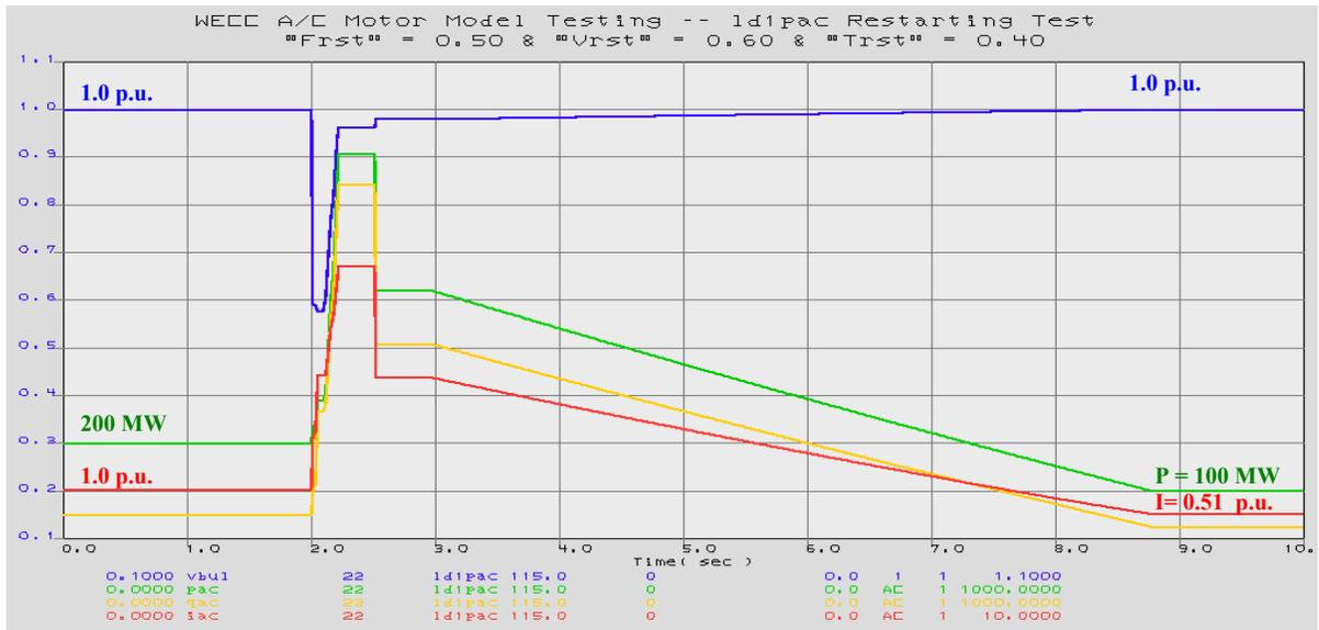
Figure 39. Restarting Fraction Test ( $Frst = 50\%$ )
