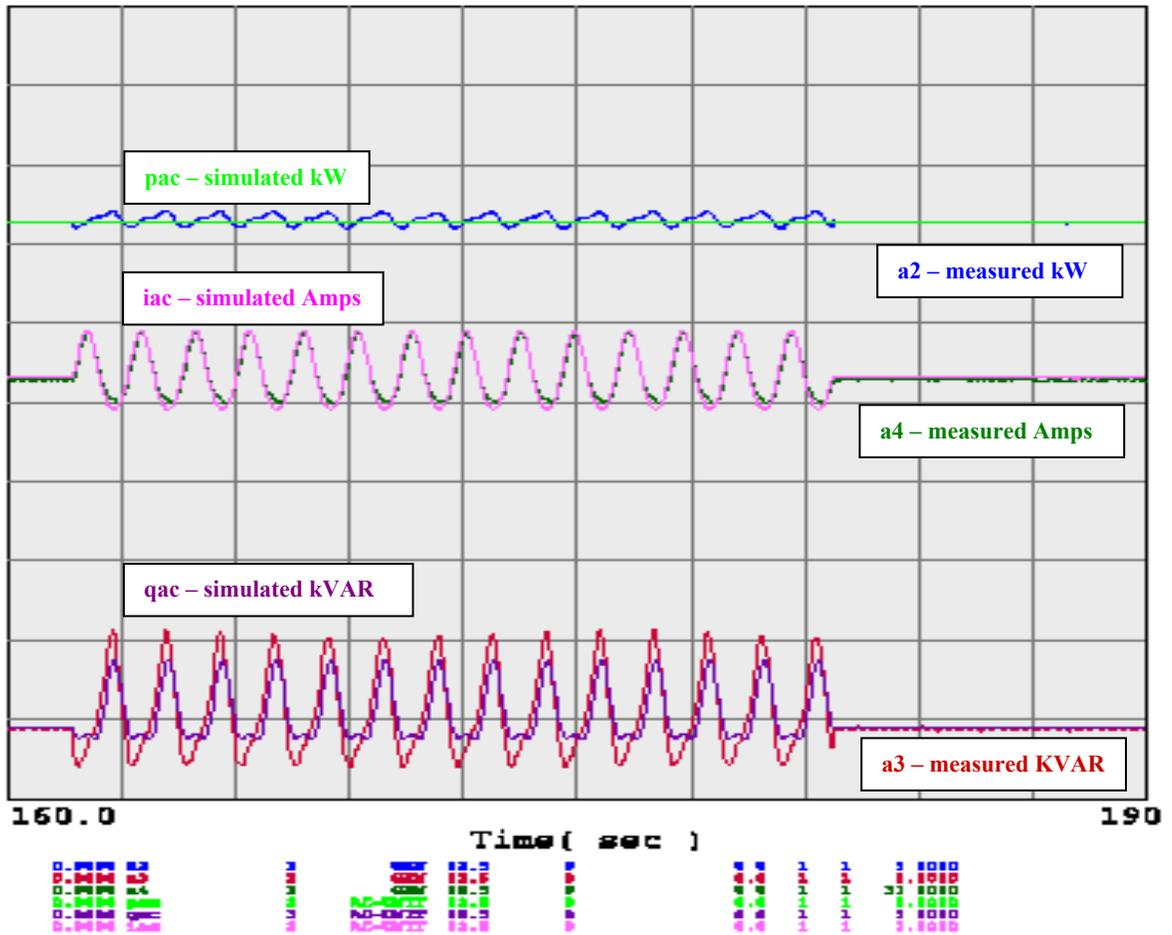
Figure 65. Voltage Oscillation at 0.7 Hz
