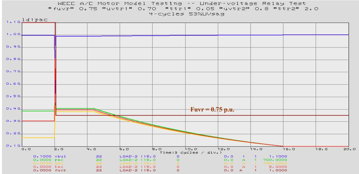
Figure 51. Fraction of UV Relay Penetration ( $F_{uvr} = 75\%$ )
