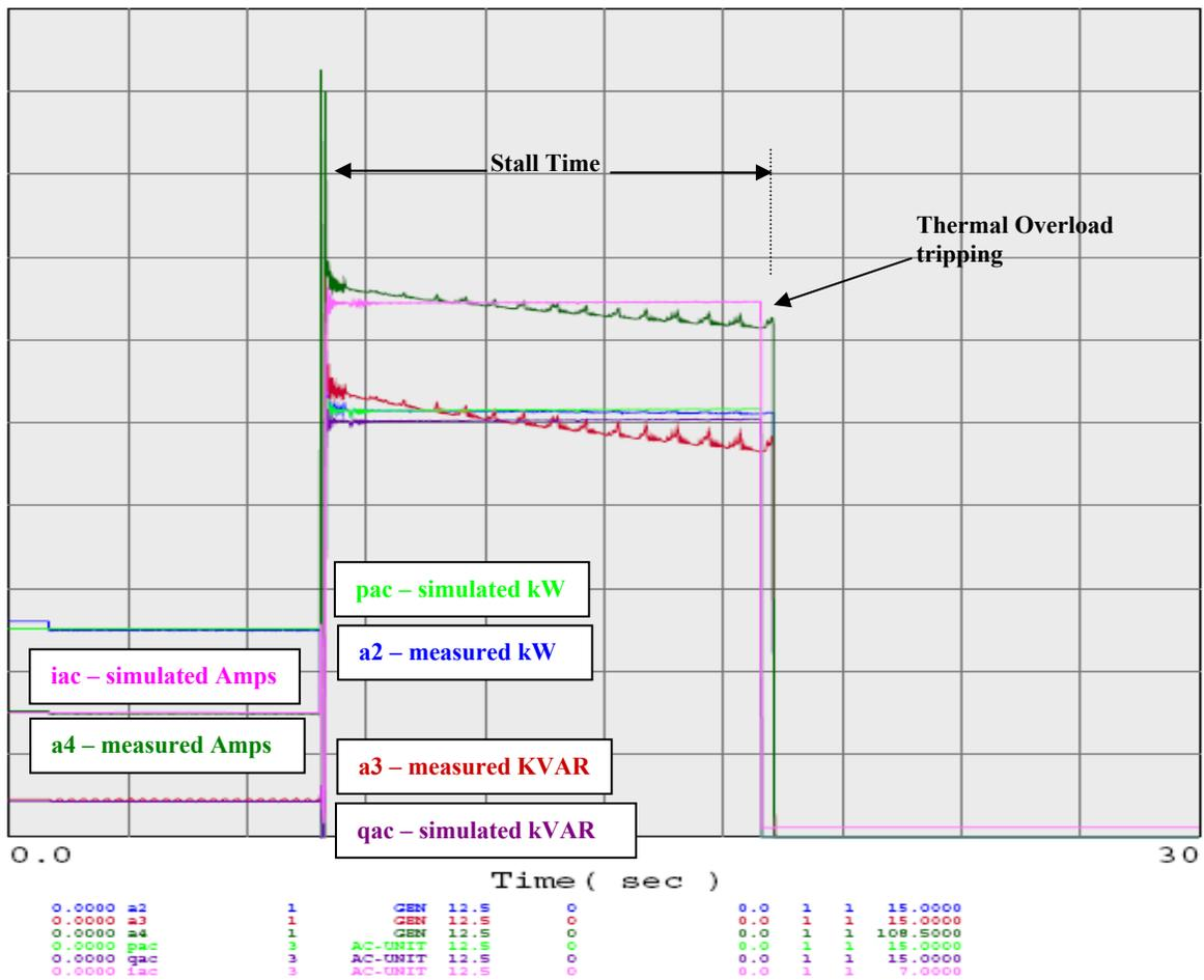
Figure 71. Voltage Sag: from 100% to 0 for 6 cycles with recovery to 70%
