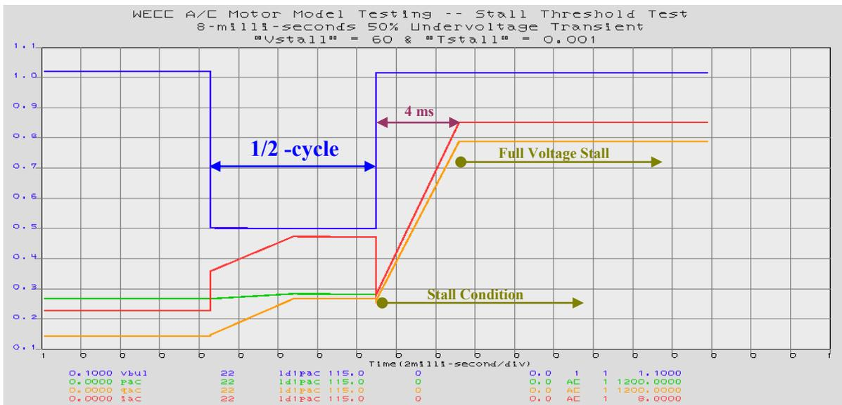
Figure 25. Stalling Response Time Test (Vstall=60% - UVsag = 50 % & 8-ms)
