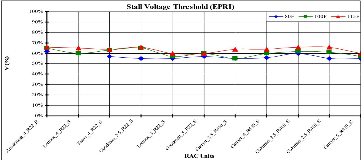
Figure 20. EPRI (APS) A/C Stalling Thresholds
