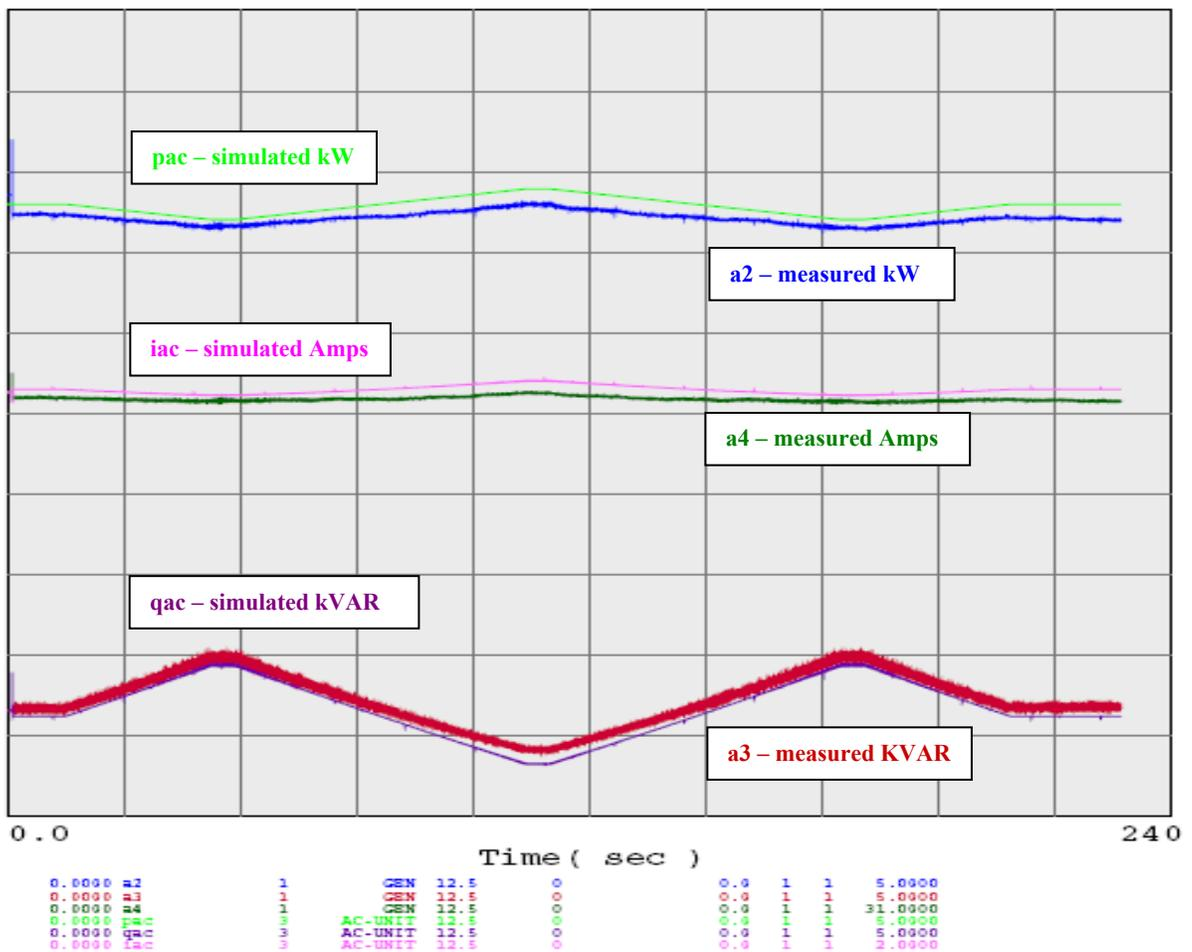
Figure 67. Frequency Ramp Test
