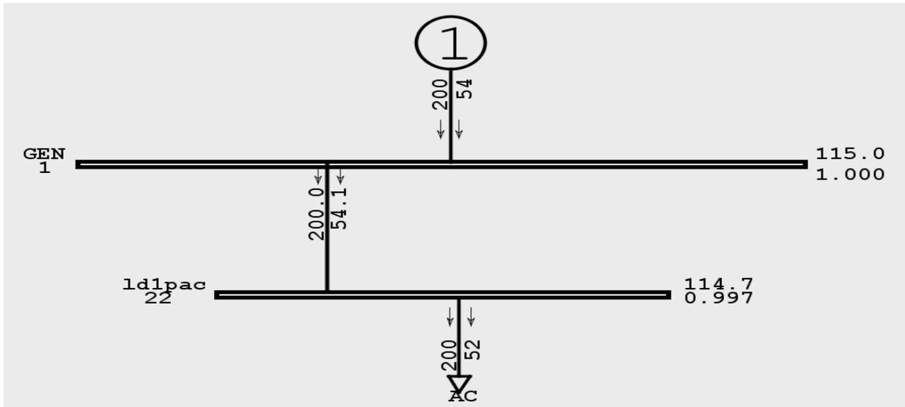
Figure 1. Air Conditioner Model Test Diagram
