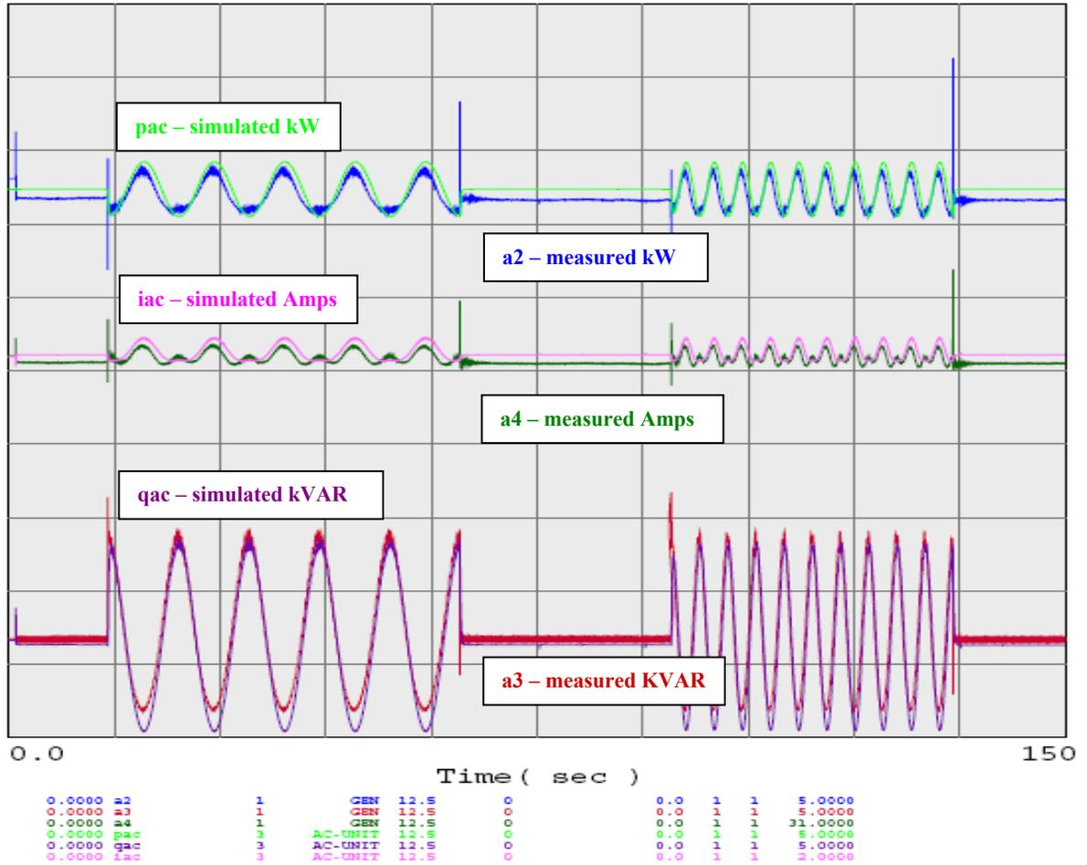
Figure 68. Frequency Oscillation at 0.1 Hz
