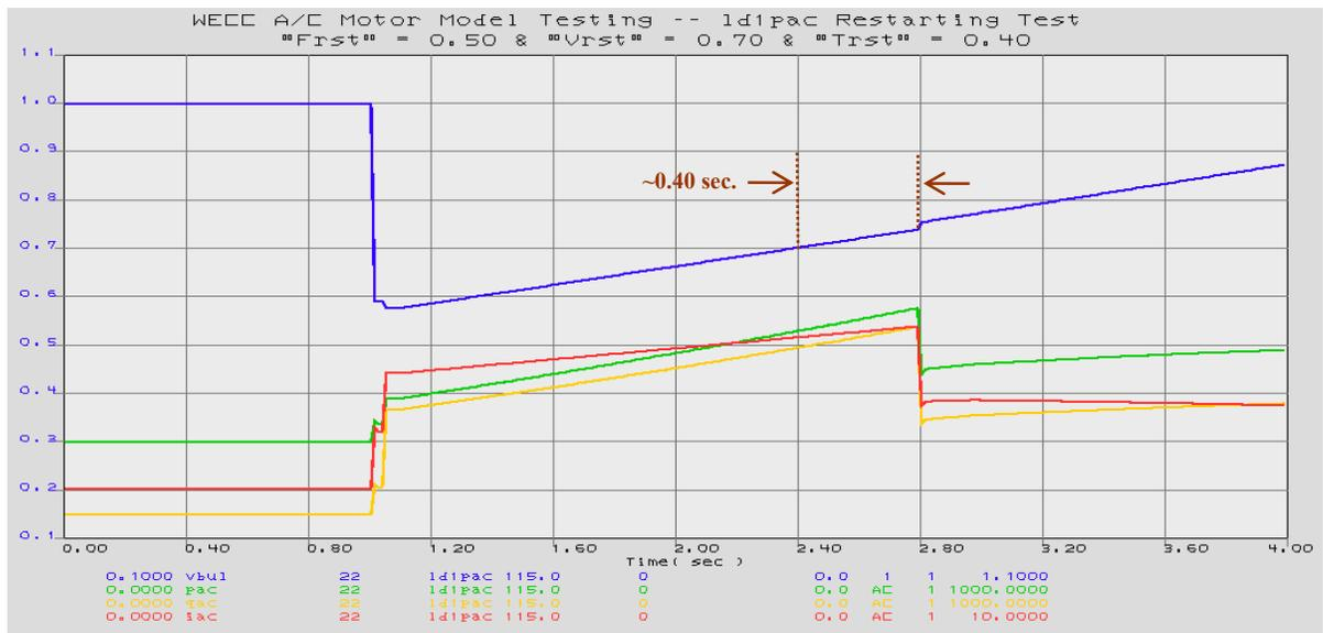
Figure 46. Restarting Delay Test ( $Trst = 0.40$ )
