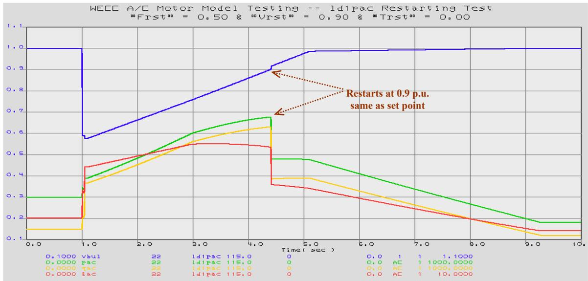
Figure 44. Restarting Voltage Test ( $V_{rst} = 90\%$ )
