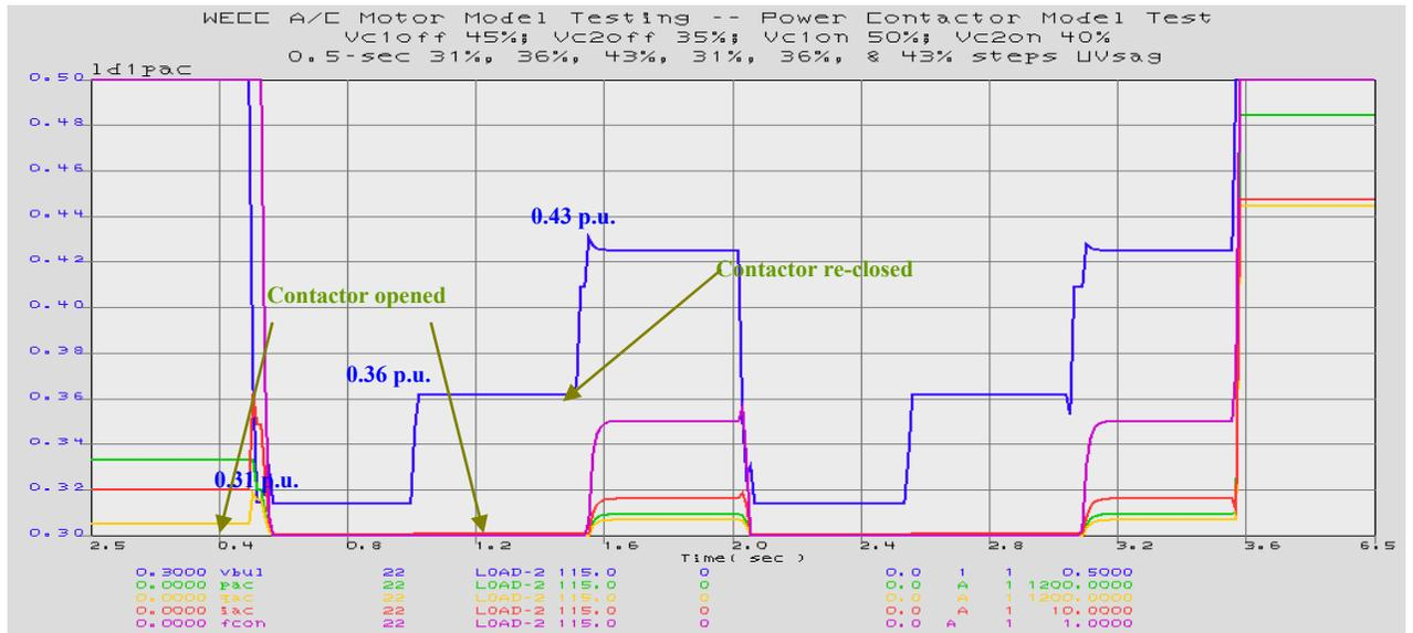
Figure 35. Contactor Second Set of Parameters ( $V_{c2off}$  and  $V_{c2on}$ ) Test
