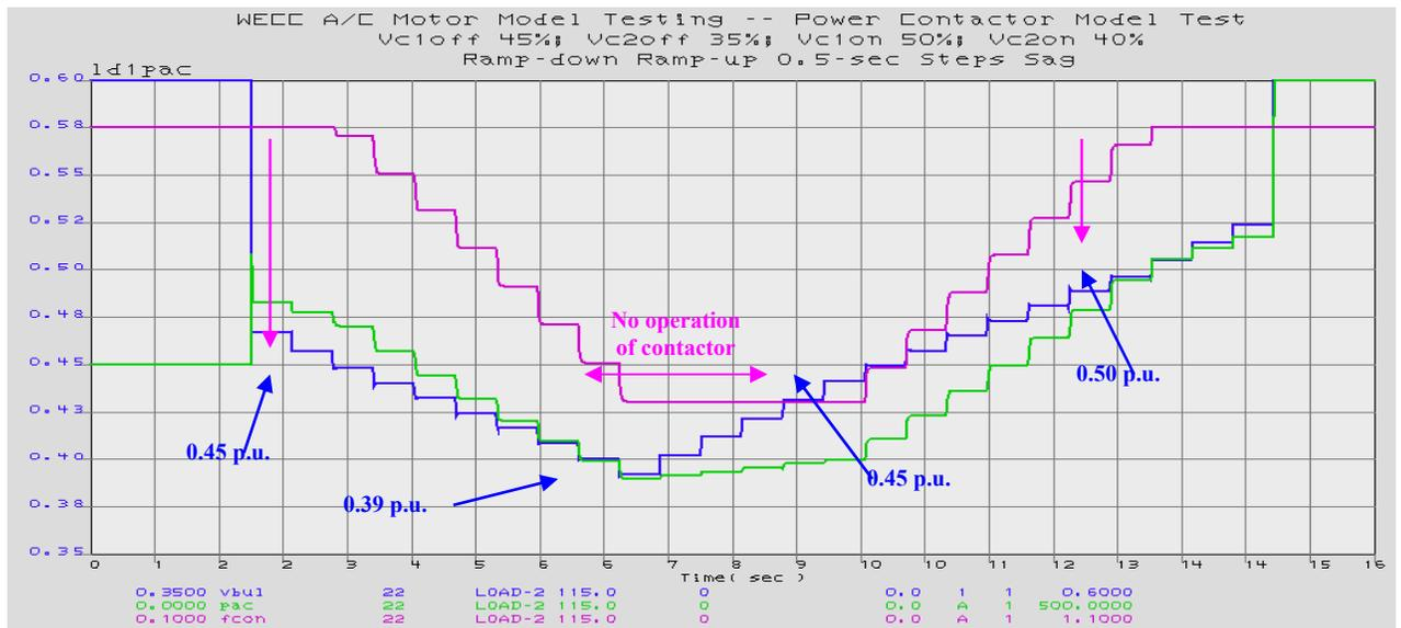
Figure 34. Contactor First Set of Parameters (*Vc1off* and *Vc1on*) Test
