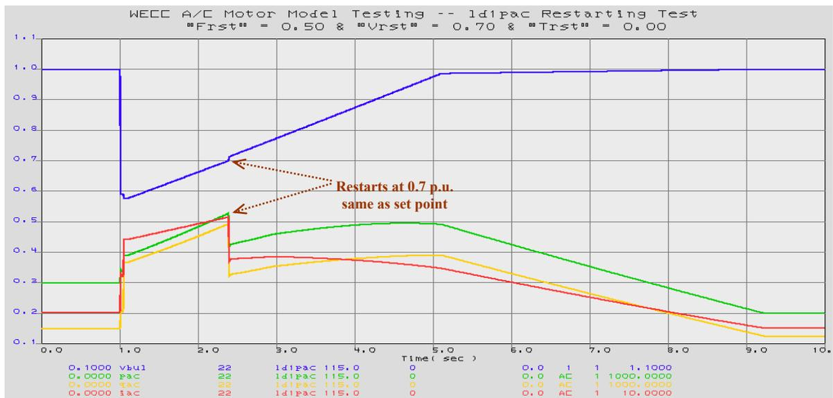
Figure 42. Restarting Voltage Test (Vrst = 70%)
