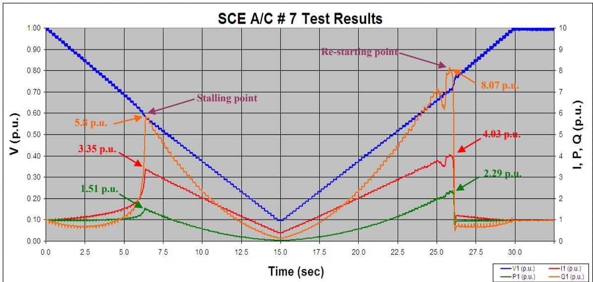
Figure 60. SCE A/C #7 Ramp-Down Ramp-Up Test Results
