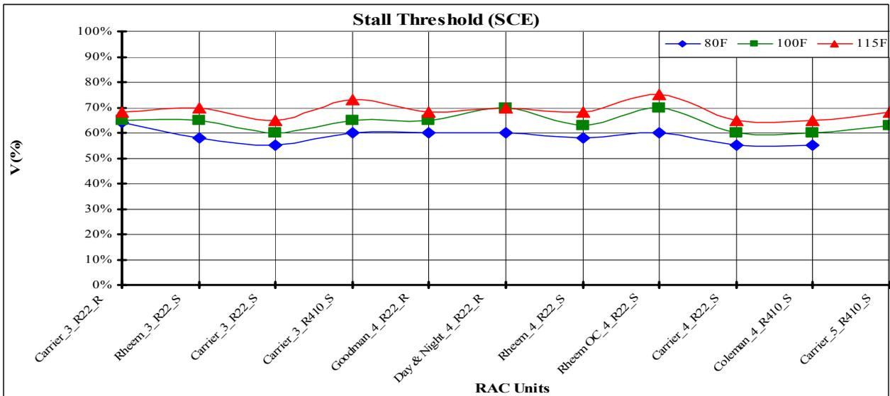
Figure 21. SCE Air Conditioner Testing
