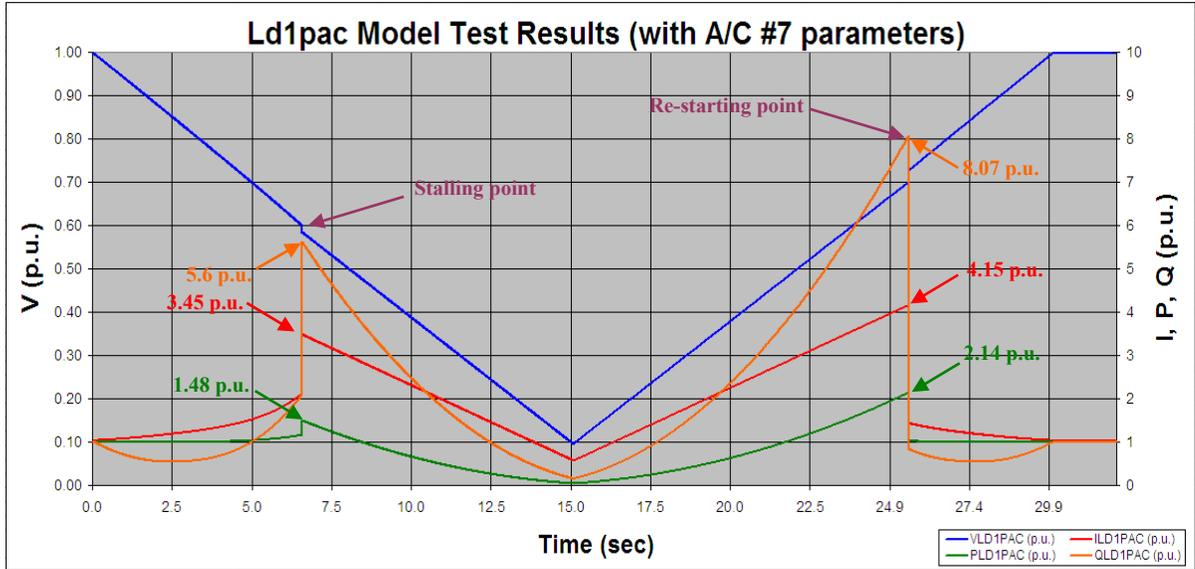
Figure 61. *Ld1pac Ramp-Down Ramp-Up Test Results (w/ A/C #7 Parameters)*
