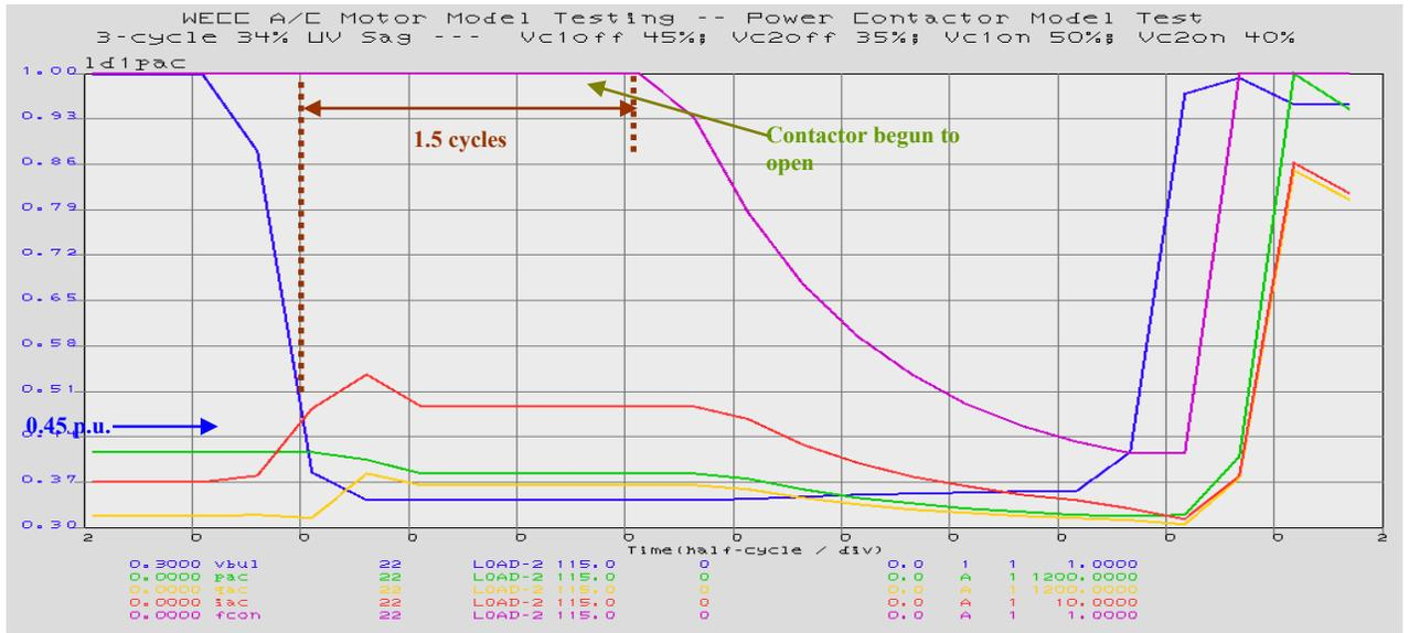
Figure 36. 3-cycles 34 UV Transient Contactor Model Test
