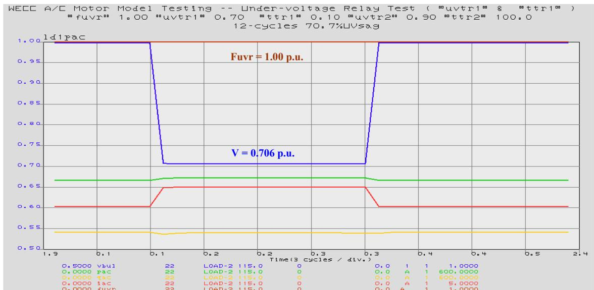
Figure 55. First UV Relay Tripping Parameters Test ( $uvtr1=70\%$  &  $ttr1=0.100$ )
