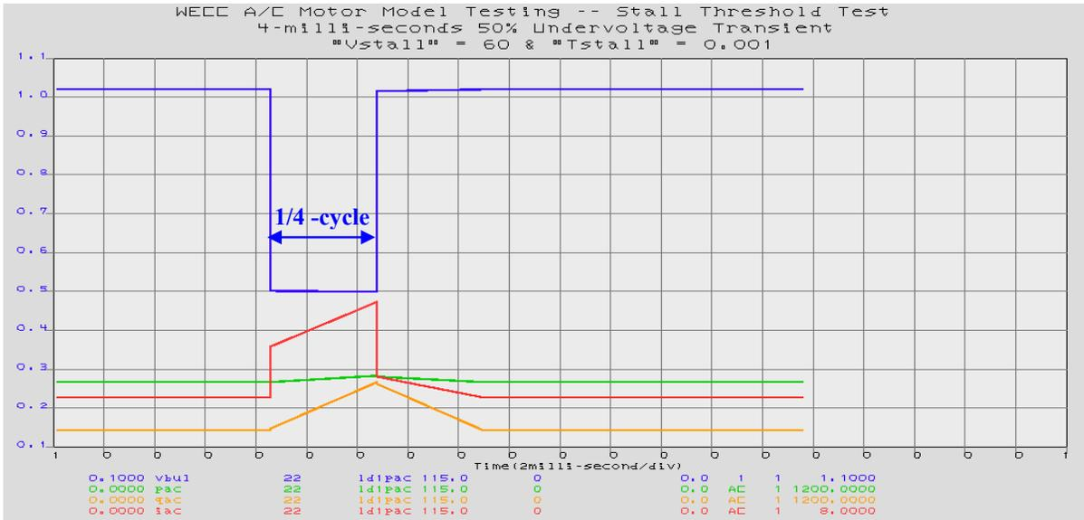
Figure 24. Stalling Response Time Test (Vstall=60% - UVsag = 50 % & 4-ms)
