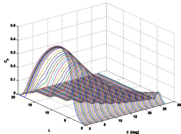
Figure 5. Wind Power  $C_p$  Curve
