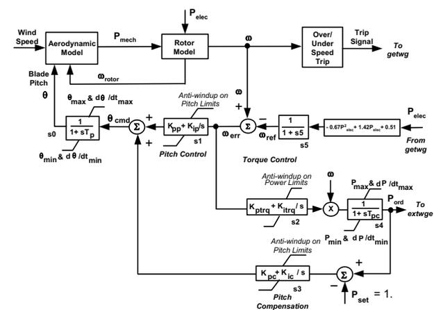
Figure 4. Wind Turbine Model Block Diagram.
