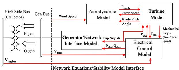
Figure 2. GE Wind Turbine Basic Dynamic Models and Data Connectivity
