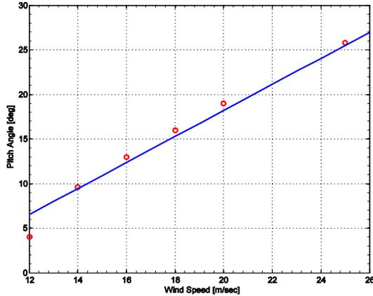
Figure 9. Pitch Angle vs. Wind Speed
