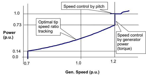
Figure 3. Power vs. Speed Steady State Curve.
