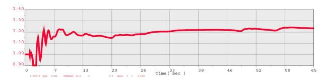
Figure 9: V/Hz measured on bus number 67908.
