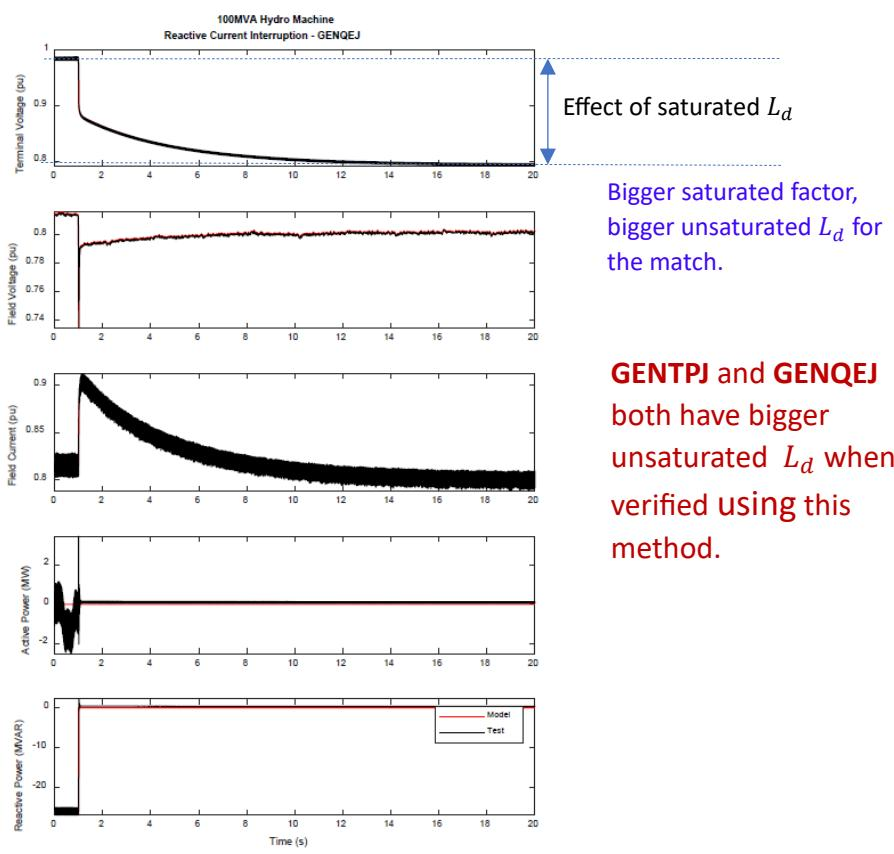
Plot above is taken from Page 13 of the Presentation for GENQEJ. The voltage drop in the D-axis load rejection test reflects the combined effect of an unsaturated  $L_d$  and the saturation effect. The application of  $K_{is}$  is to universally increase the degree of saturation even in under-excited operating conditions. Consequently, the unsaturated  $L_d$  verified using GENTPJ and GENQEJ through this d-axis load rejection is bigger than other second-order synchronous machine models.
