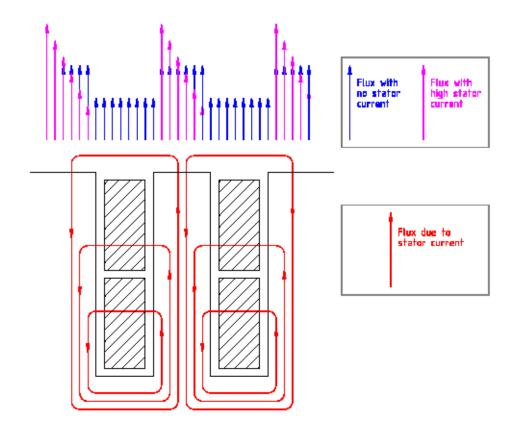
Stator current distorts the flux distribution in many parts of the machine. For example, in this illustration the flux profile across the center tooth is uniform when there is no stator current (blue) and is distorted when stator current is present (magenta). Stator current increases the degree to which saturation affects the flux crossing the air gap.
