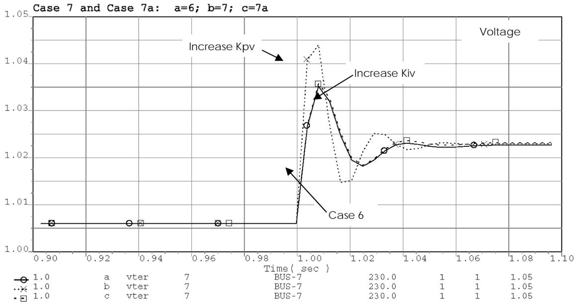
**Figure A-16. Case 7 simulation result compared to Case 6; voltage.**
