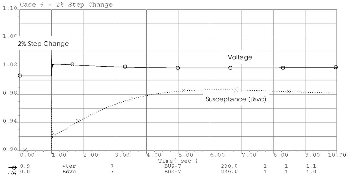
**Figure A-14. Case 6 simulation result; voltage and susceptance.**
