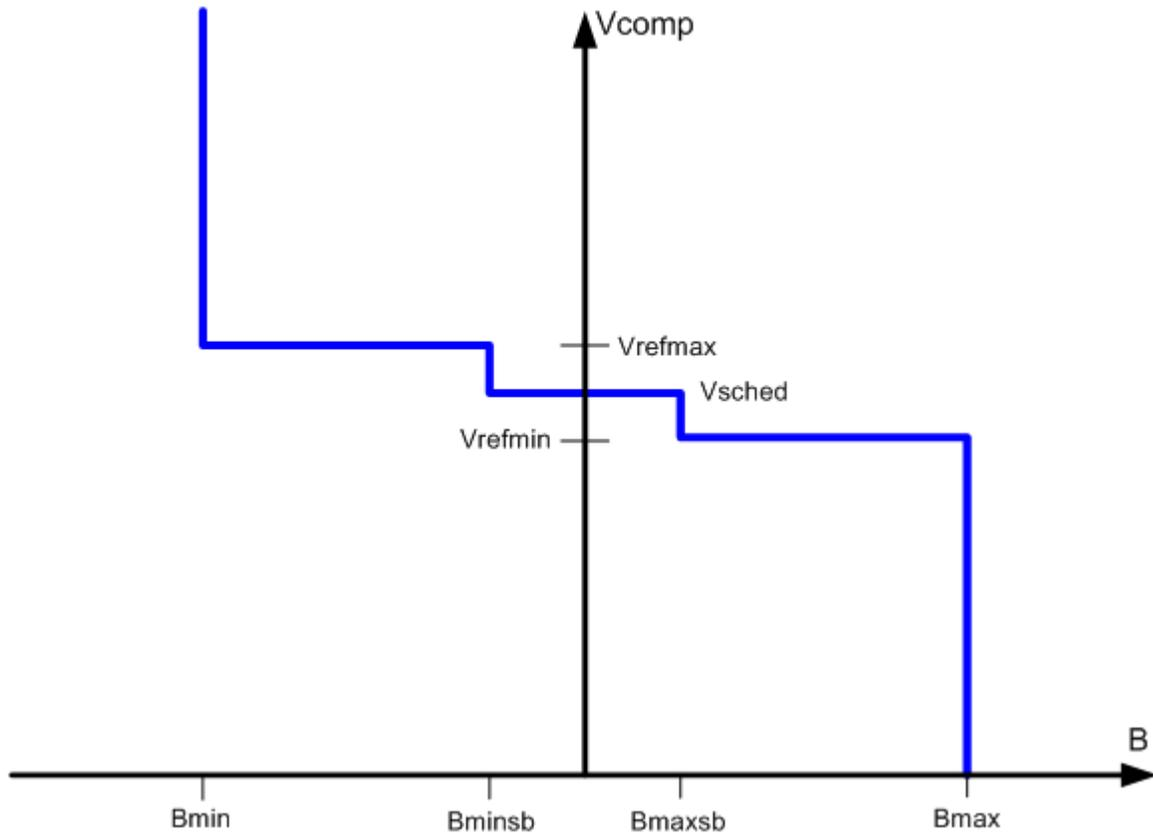
**Figure 2-17: Steady-state powerflow boundary conditions of the SVC slow-susceptance solution.**
