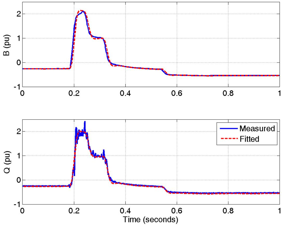
**Figure 3-4: Measured and simulated reactive power output and susceptance response of a transmission SVC installation. Response is to an unbalanced fault.**
