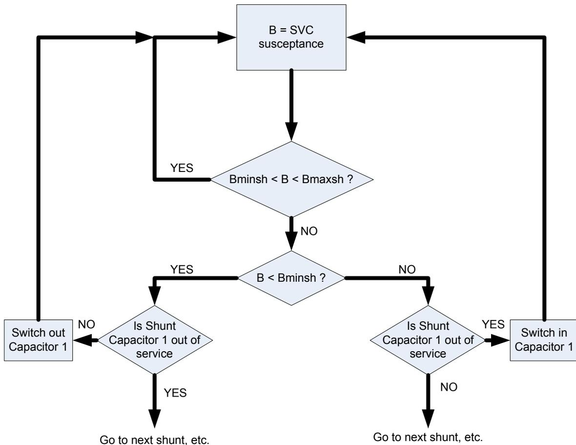
**Figure 2-16: Flow chart for the MSS switching logic.**
