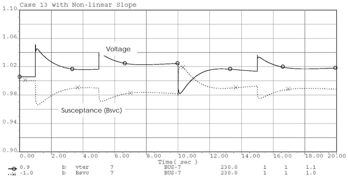
Figure A-28. Case 13 simulation result with non-linear slope activated.
