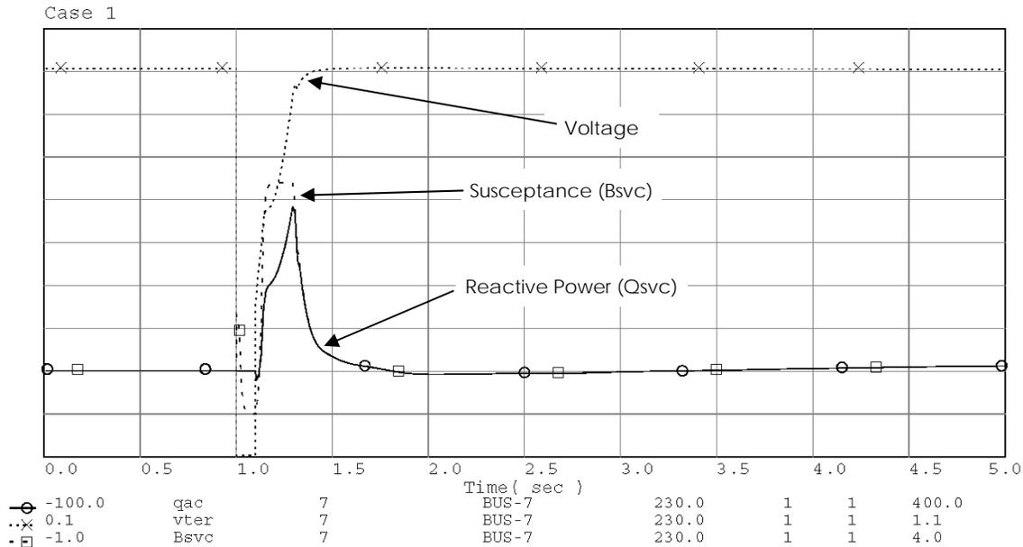
Figure A-2. Case 1 simulation result; voltage, susceptance, and reactive power.
