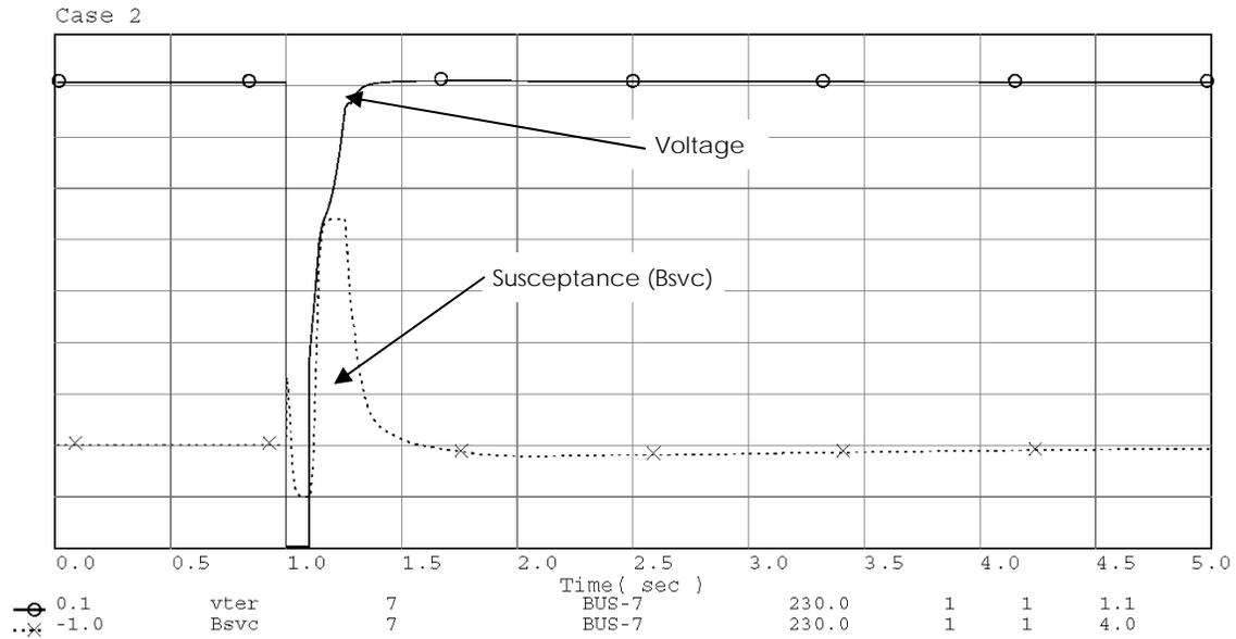
Figure A-6. Case 2 simulation result; voltage and susceptance.
