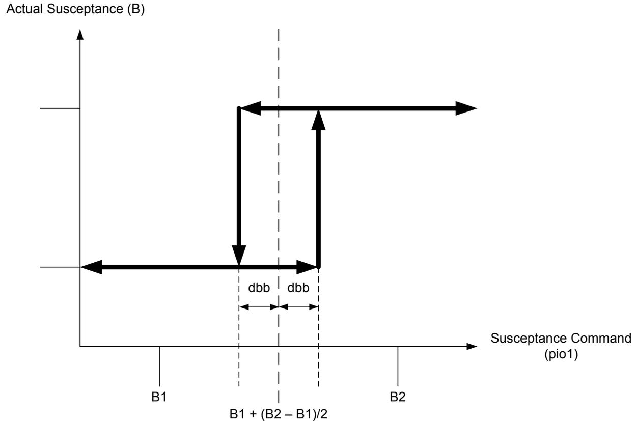
**Figure 2-11: Switching from one susceptance level to the next.**
