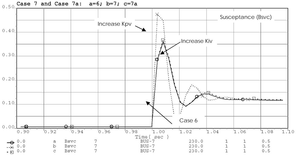
**Figure A-17. Case 7 simulation result compared to Case 6; susceptance.**
