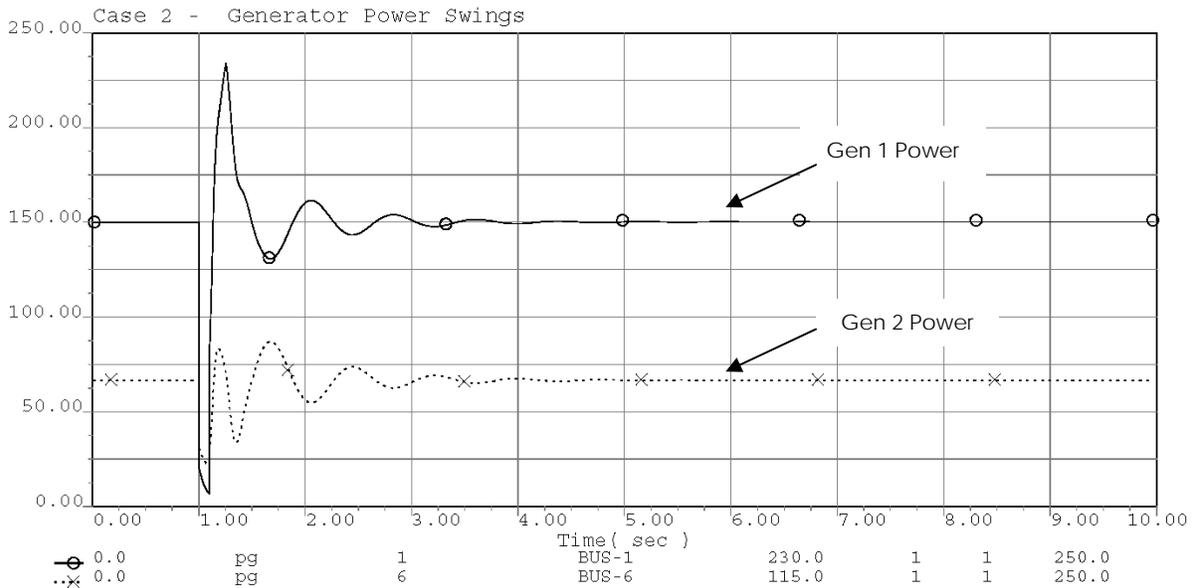
Figure A-7. Case 2 simulation result; power swings
