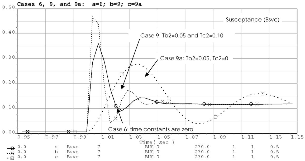
Figure A-21. Case 9 and 9a simulation results compared to Case 6; susceptance.
