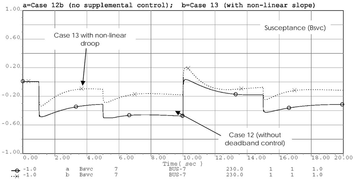
**Figure A-30. Susceptance for Case 13 simulation compared to Case 12b (with no deadband control).**
