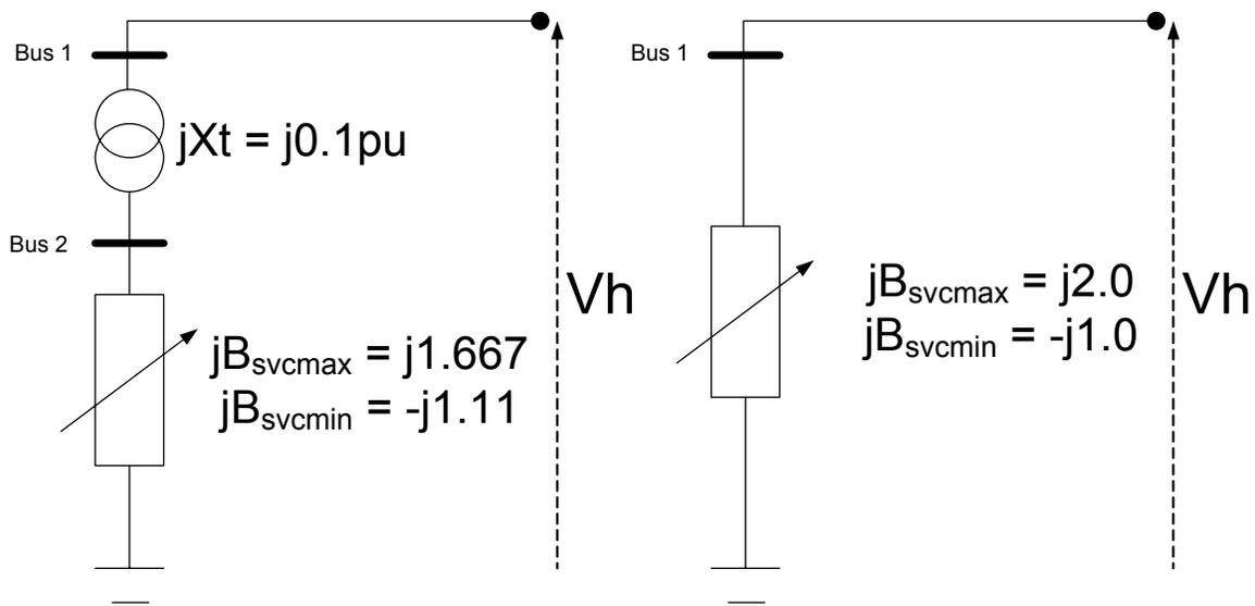
**Figure B-2: SVC modeled with and without the coupling transformer.**
