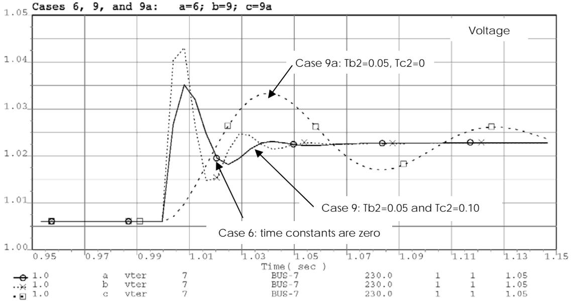
Figure A-20. Case 9 and 9a simulation results compared to Case 6; voltage.
