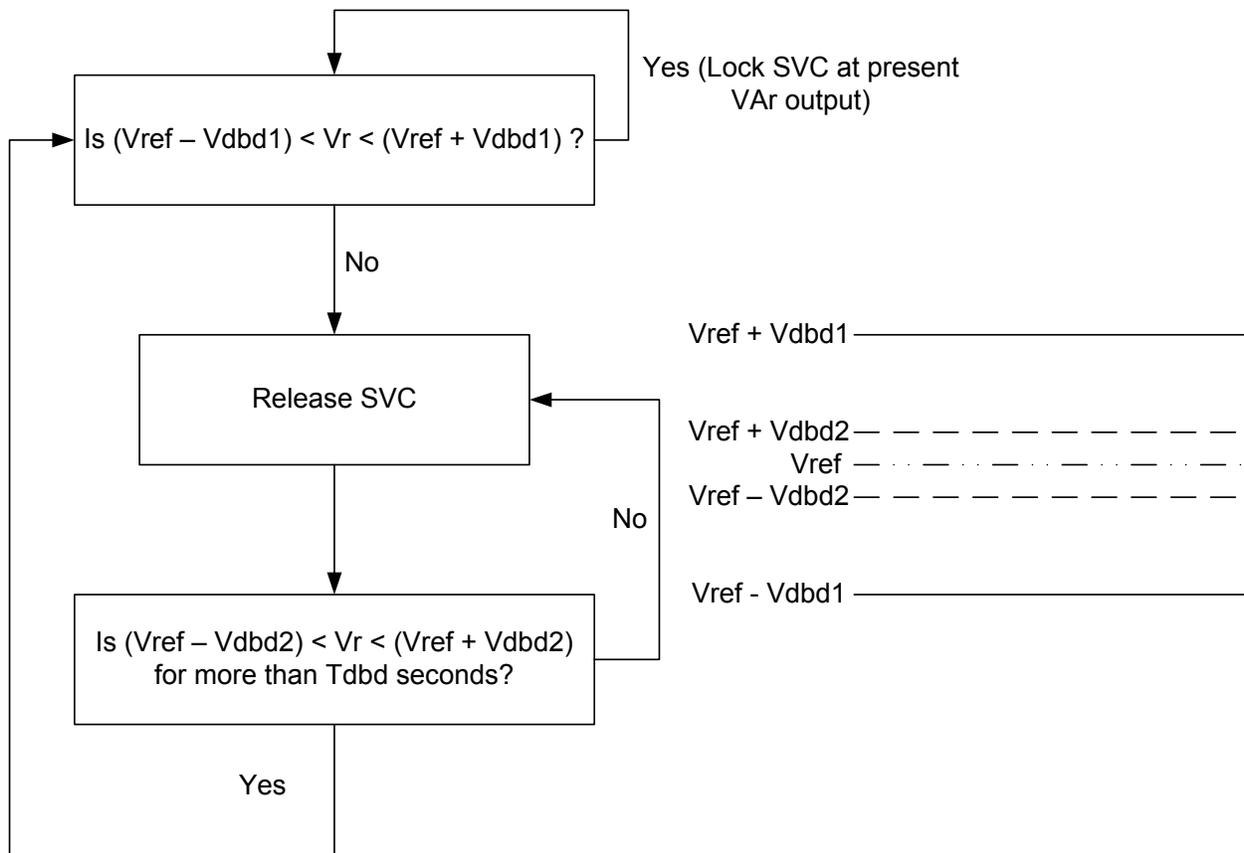
**Figure 2-6: Deadband control logic.**
