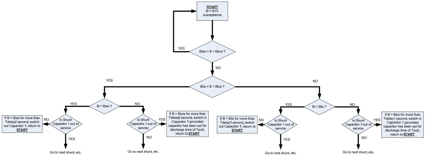
**Figure 2-9: MSS switching logic**
