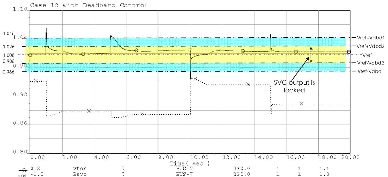
Figure A-24. Case 12 simulation result – with deadband control activated
