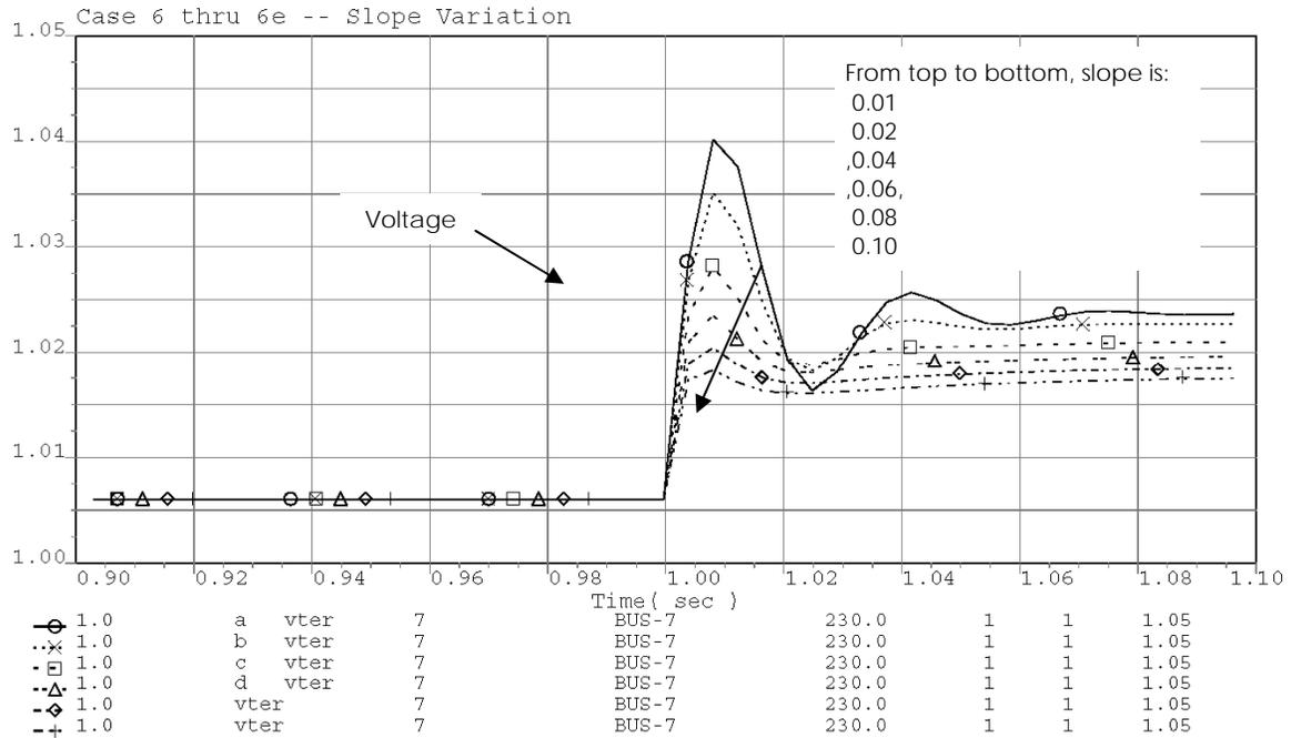
Figure A-15. Impact of slope variation on voltage response.
