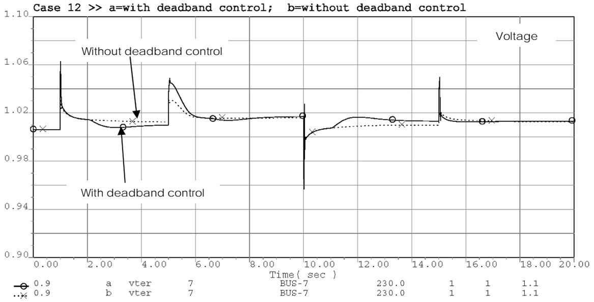
**Figure A-27. Case 12 – comparing regulated bus voltage with and without deadband control**
