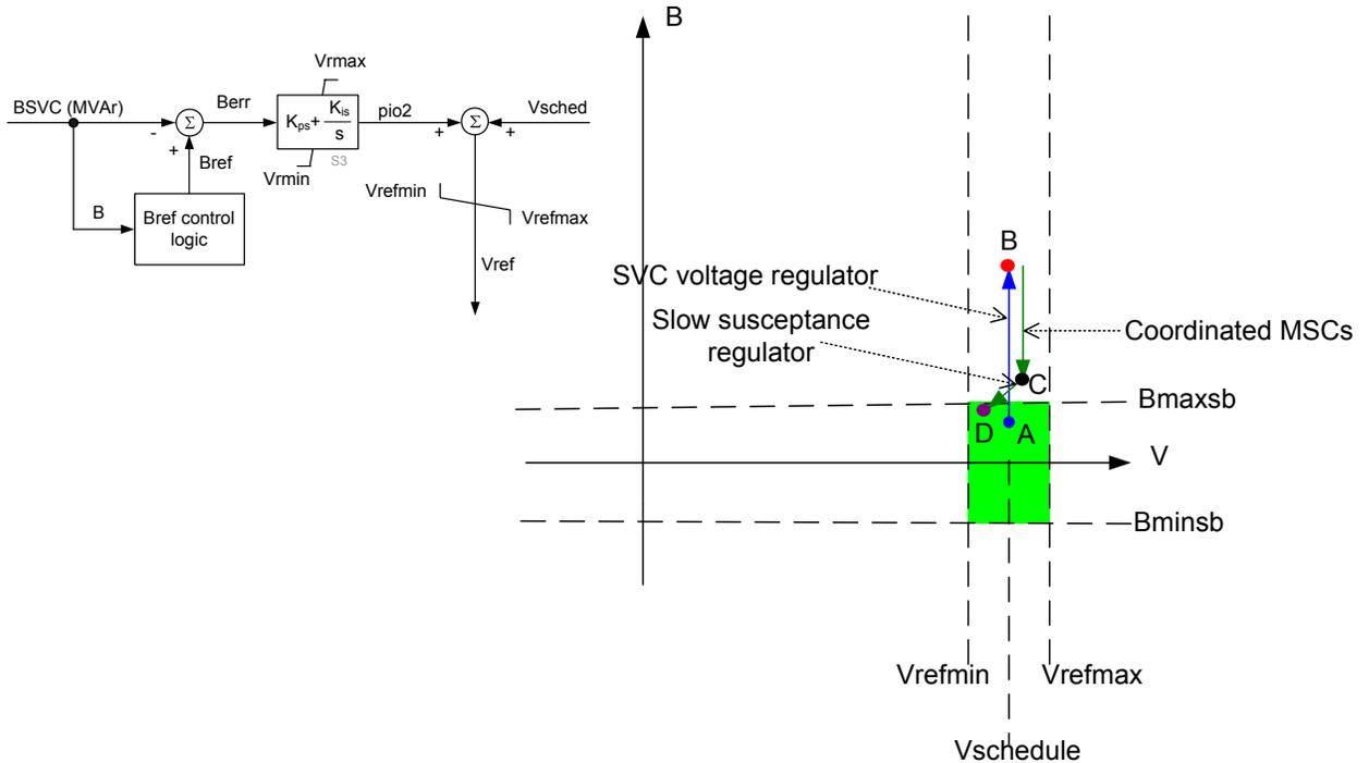
**Figure 2-18: Functioning of the slow-susceptance regulator.**
