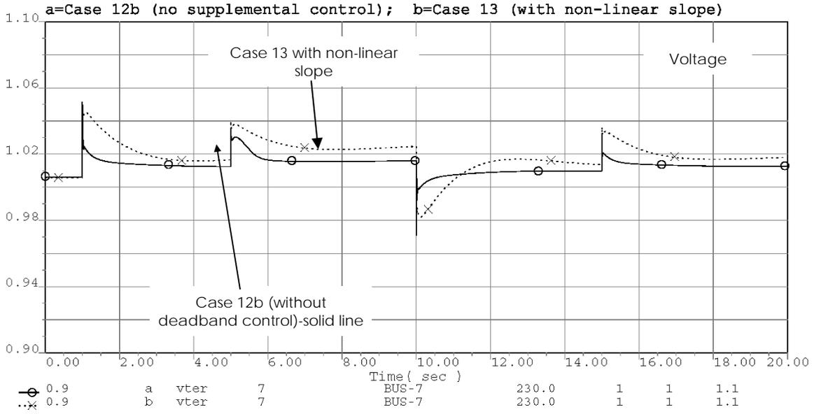
**Figure A-29. Voltage for Case 13 simulation compared to Case 12b (with no deadband control).**
