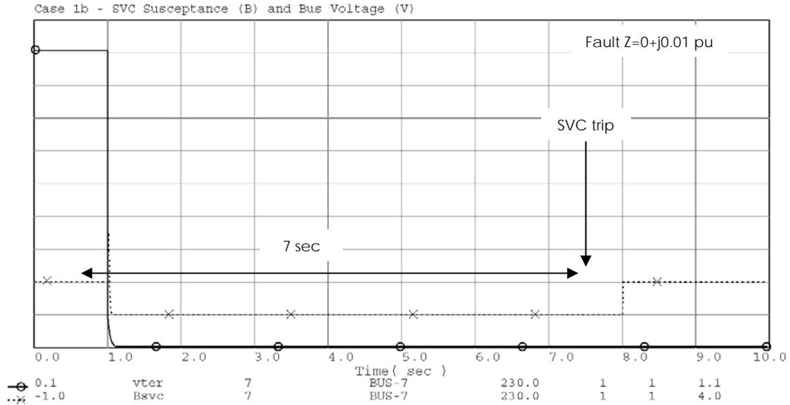
Figure A-4. Case 1b simulation result; undervoltage trip UV2
