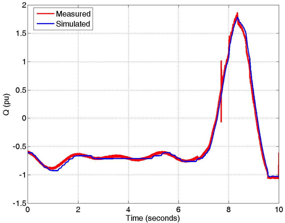
**Figure 3-3: Measured and simulated reactive power output response of a transmission SVC installation. Response is to a WECC-wide event.**
