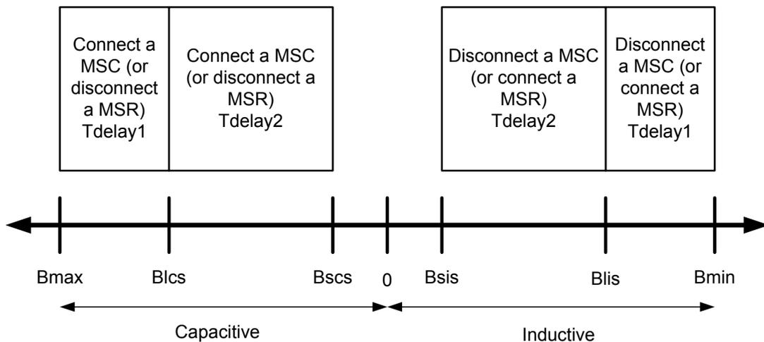
**Figure 2-7: Settings for the MSS switching logic based on SVC susceptance.**
