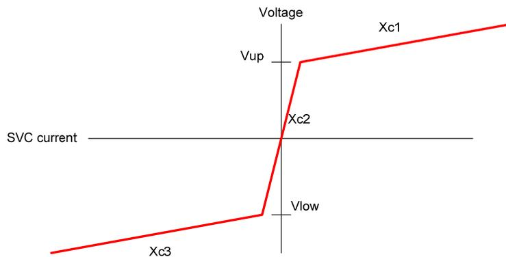
Figure A-28 illustrates the operation of the non-linear slope control function, with Figures A-29 and A-30 illustrating the comparison between Case 13 and Case 12 (without deadband control)
