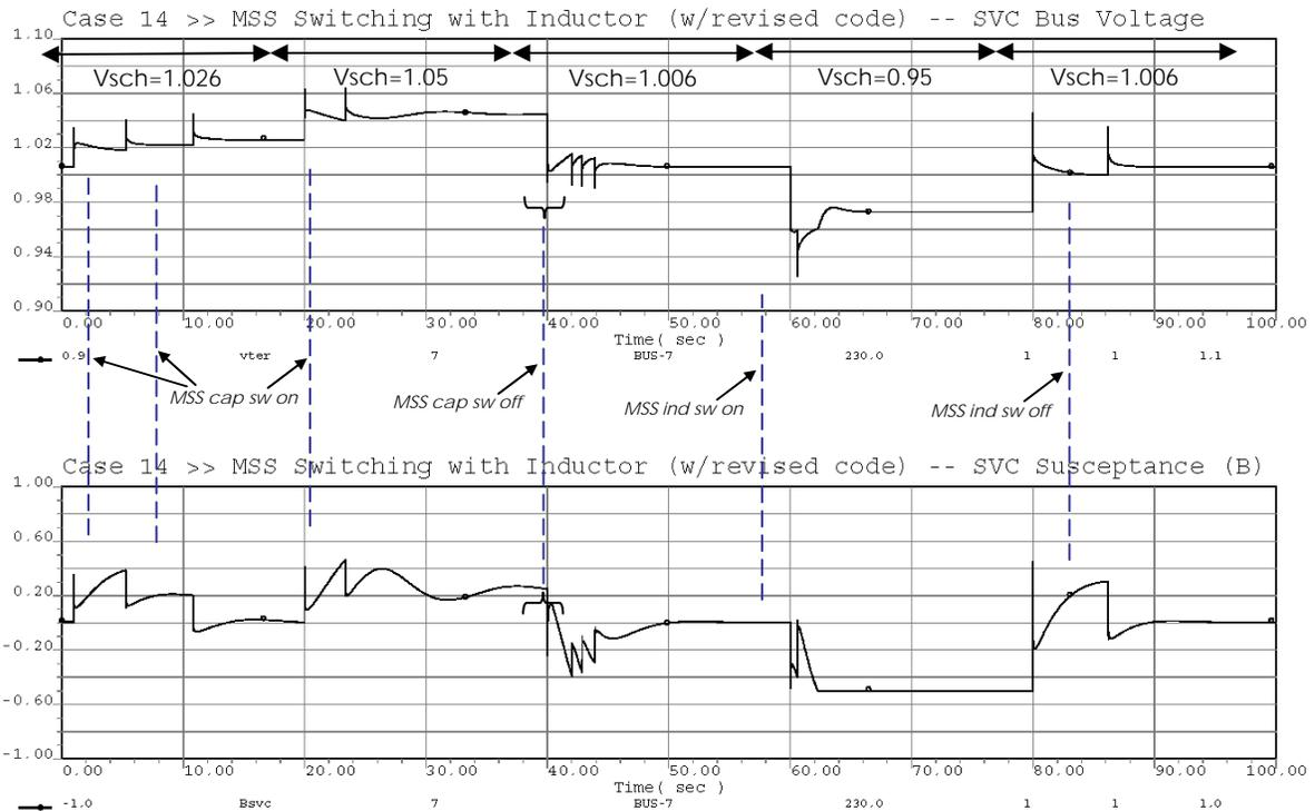
**Figure A-32. Case 14 simulation result with Inductor switching.**
