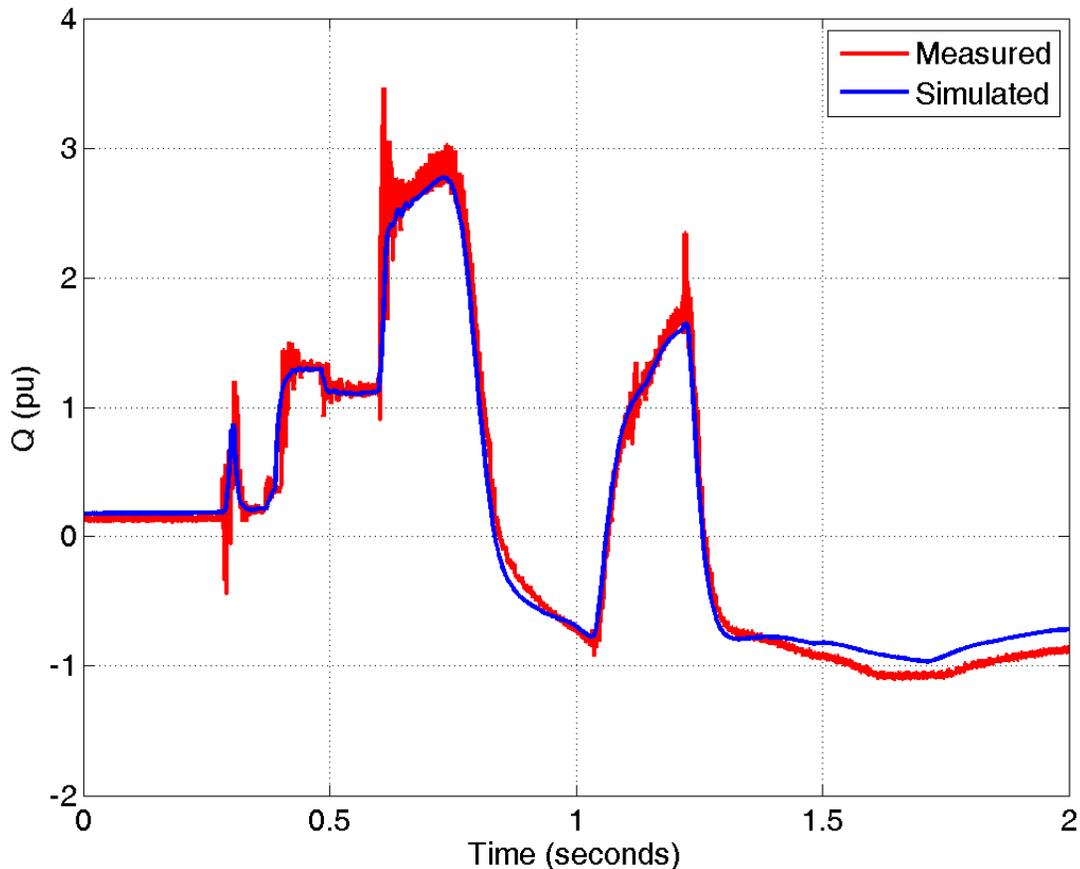
**Figure 3-2: Measured and simulated reactive power output response of a transmission SVC installation. Response is to a delayed clearing of a transmission fault (see [\[8\]](#) for a description of the event).**
