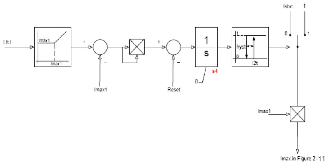
Figure 2-14: I2t short-term rating logic (figure reproduced from [9]).
