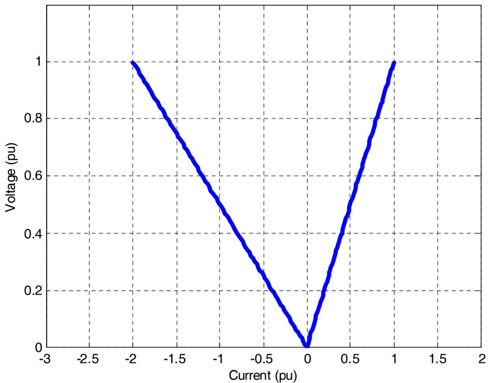
**Figure B-3: SVC VI characteristic from 0 to 1 pu voltage (ideal case, not showing protection and under/overvoltage strategies).**
