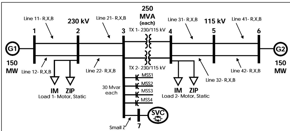
**Figure A-1. Simplified One-Line for Test System Model**
