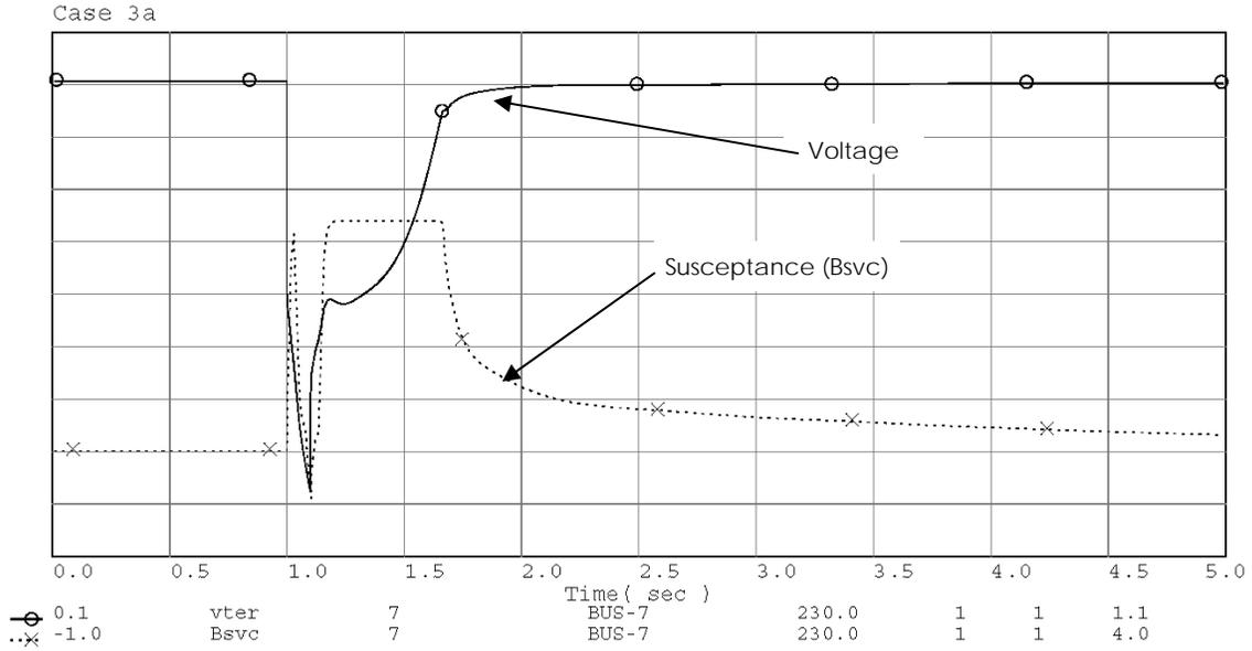
**Figure A-10. Case 3 simulation result; voltage and susceptance.**
