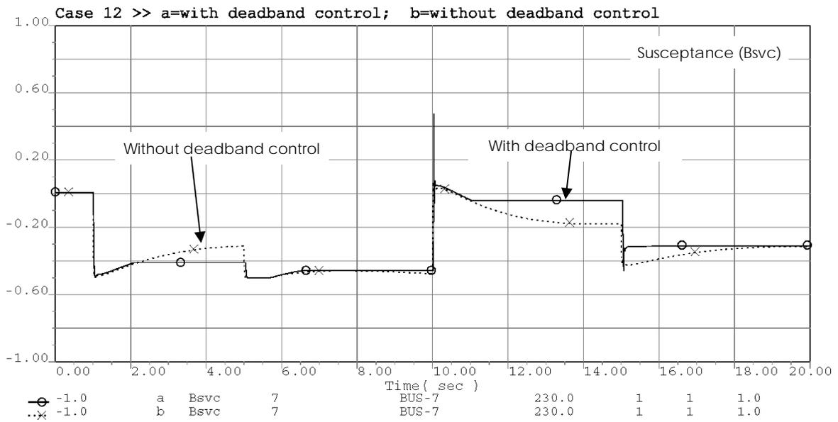
Figure A-26. Case 12 – comparing Bsvc with and without deadband control.
