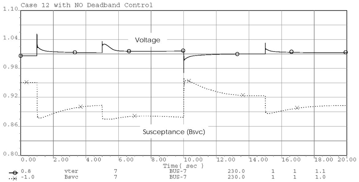
Figure A-25. Case 12 simulation result – without deadband control activated
