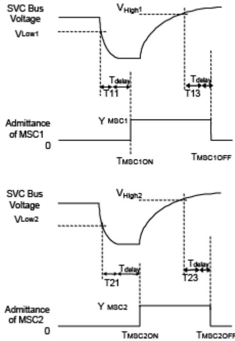
Figure 2-4: Voltage-Based MSS switching (reproduced from [\[11\]](#) IEEE© 2006)
