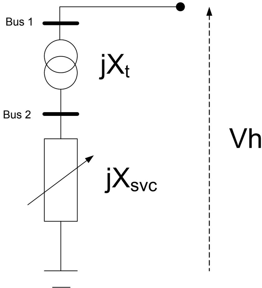
Figure B-1: SVC and coupling transformer.
