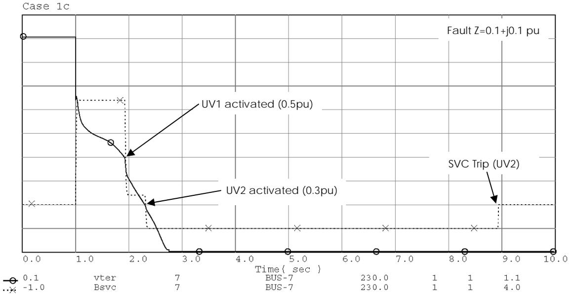
**Figure A-5. Case 1c simulation result; undervoltage trip UV1 and UV2**
