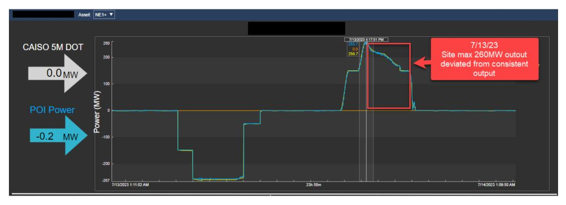
First day of scheduled BESS 260MW discharge, inverters began tripping and reducing output
