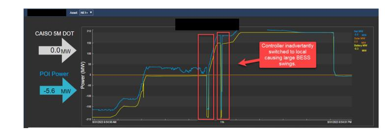
Challenges with developer integrator on BESS tuning testing. Issues with large BESS swings while tuning available BESS units to a consistent output.
