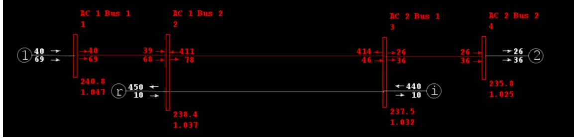
Figure 10: Simple test system for VSC-HVDC model.
