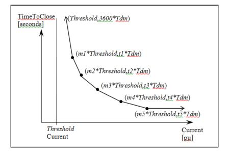
For the equation-based relay models, instead of using a piece-wise linear curve, an equation as described in IEEE, IEC, SEL or other standards is used. The task forces' discussions with many relay engineers from within member utilities indicates that some relay engineers are most accustomed to specifying overcurrent relays using these types of equations.
