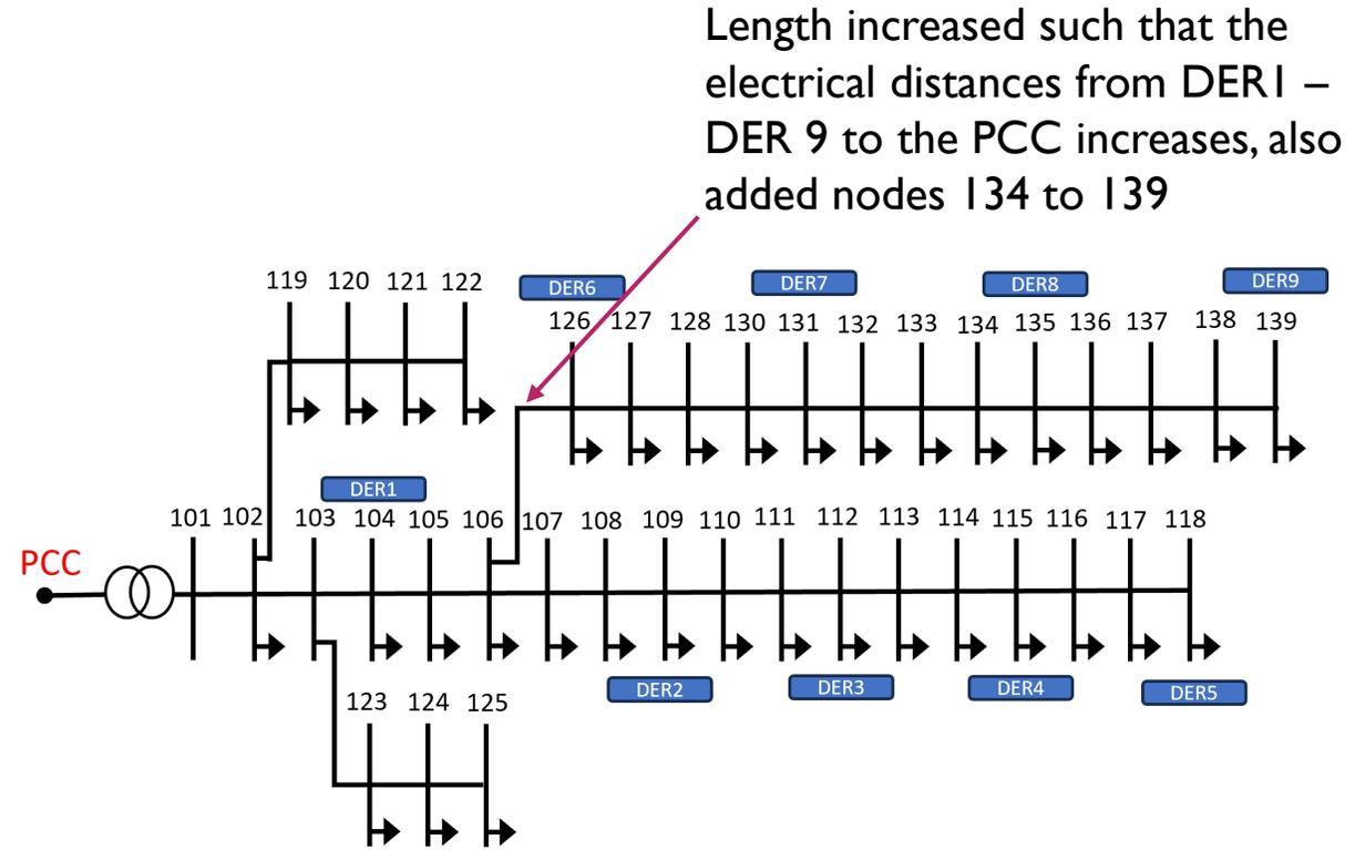
Length increased such that the electrical distances from DER1 – DER 9 to the PCC increases, also added nodes 134 to 139
