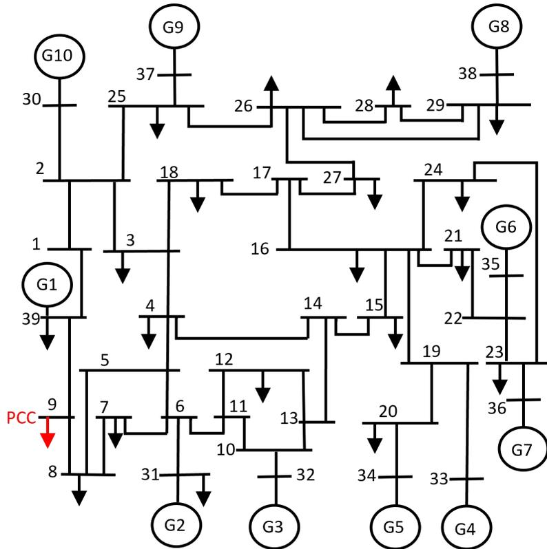
(a): IEEE 39-bus transmission system as bulk power system (Phasor model)
