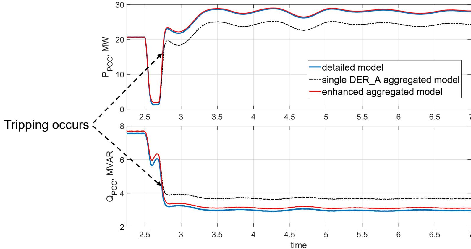
**Responses at the PCC for different DER modeling for a fault at Bus 8.**
