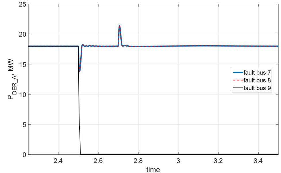
Fails to match the total DER output for any partial tripping (Faults at buses 7 and 8).
