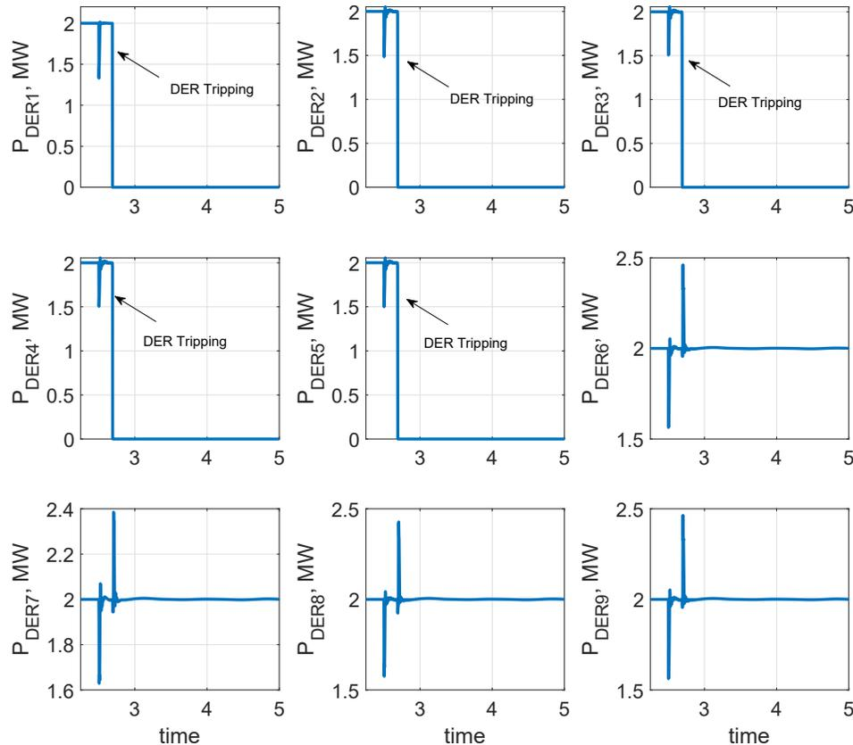
Power output of nine DERs following the 3-phase fault at bus 8.
