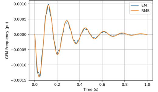
**RMS models may fail to capture some faster modes and may have a different response depending on various parameters**
