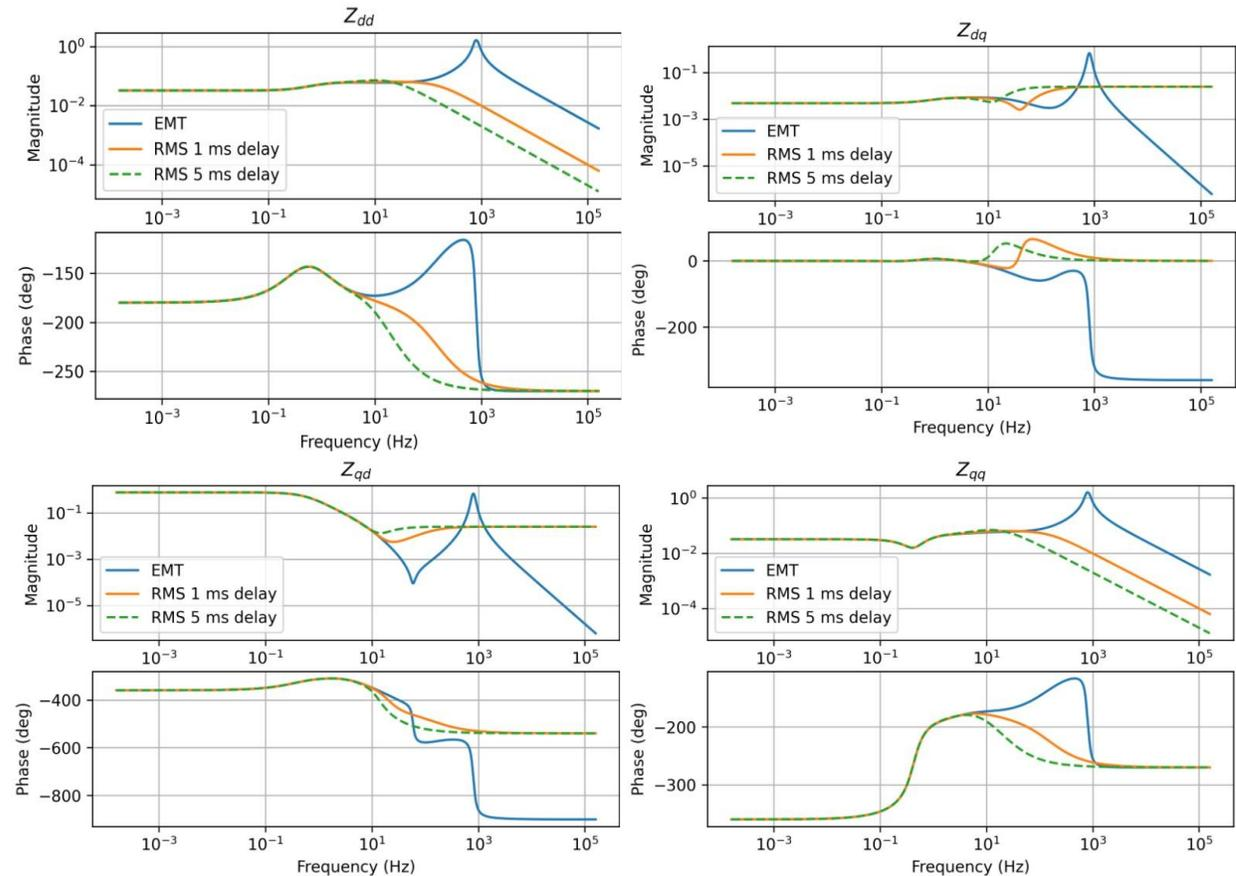
Large differences in higher frequency range, depends on RMS voltage source delay
