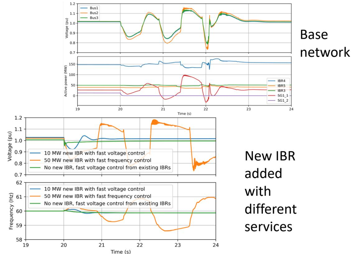
**For this disturbance, fast voltage response from existing IBRs is sufficient to ensure stable response**
