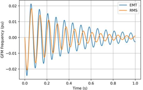
Impact of decreasing droop time constant – 0.02s left vs 0.01s right: Interactions of swing mode with dynamics only captured by EMT model
