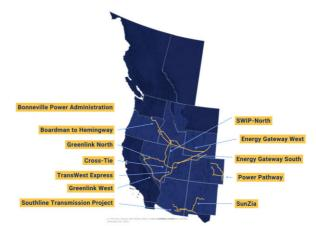
Greenlink West: 525kV line spanning 350 miles from Las Veg as, Nevada, to Yerington, Nevada. Construction is expected to begin in early 2025, with the line in service by spring 2027 Greenlink North: 525-kV line running from Ely, Nevada, to Yerington, Nevada. Expected to be in service in late 2028.
