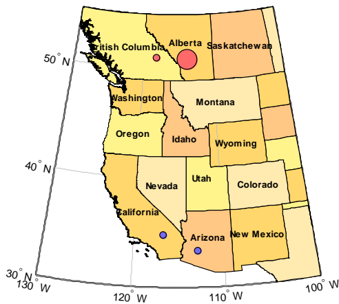
Fig. 10: Map of NS Mode A shape from Fig. 9. Red circles oscillate against blue; circle diameter is proportional to mode-shape magnitude. Alberta weakly connected.
