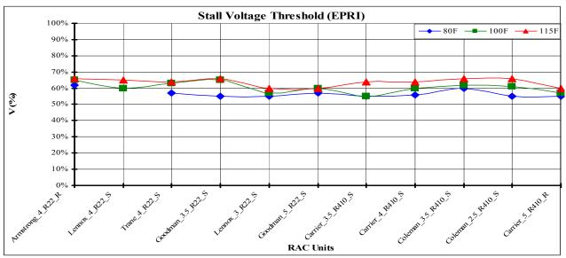
Figure 20. EPRI (APS) A/C Stalling Thresholds
