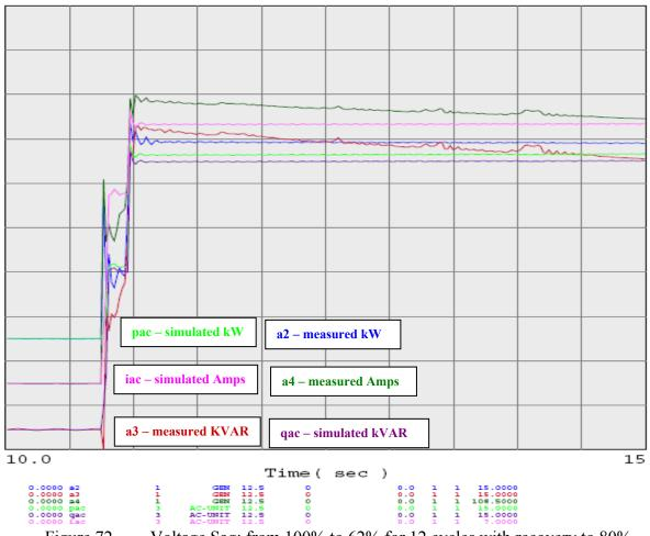
Figure 72. Voltage Sag: from 100% to 62% for 12 cycles with recovery to 80%
