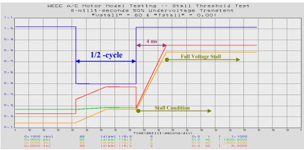
Figure 25. *Stalling Response Time* Test (Vstall=60% - UVsag = 50 % & 8-ms)
