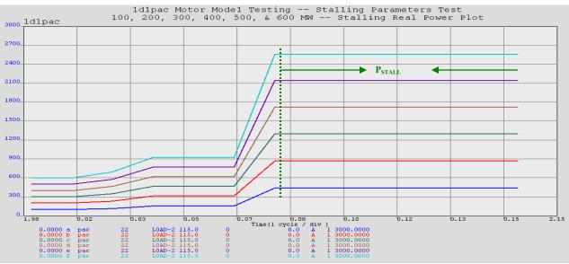
Figure 77. *Ld1pac* Model Parameters Test (Stall Real Power Plot)
