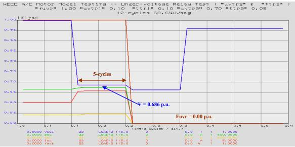
Figure 57. Second UV Relay Tripping Parameters Test (*uvtr2*=0.70% & *ttr2*=0.05)
