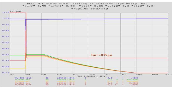
Figure 51. Fraction of UV Relay Penetration (Fuvr = 75%)
