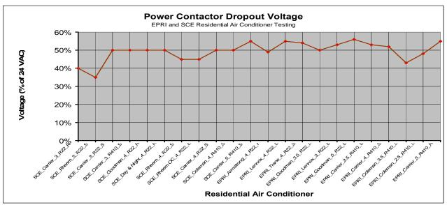
Figure 33. Power Contactor Dropout Voltages
