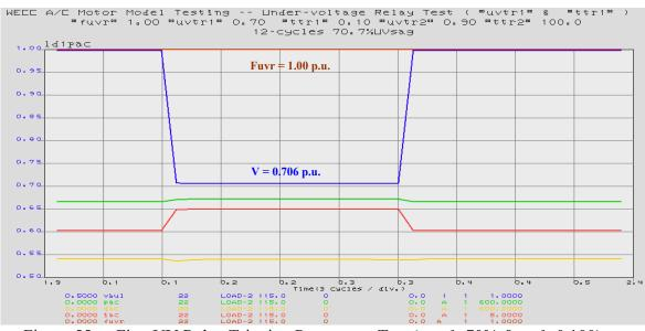
Figure 55. First UV Relay Tripping Parameters Test (*uvtr1*=70% & *ttr1*=0.100)
