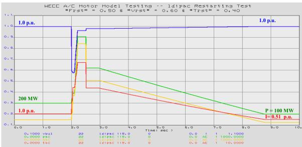
Figure 39. Restarting Fraction Test (*Frst* = 50%)
