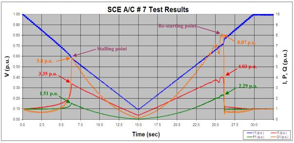
Figure 60. SCE A/C #7 Ramp-Down Ramp-Up Test Results
