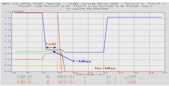
Figure 52. First UV Relay Tripping Parameters Test (uvtr1=0.70 & ttr1=0.00)
