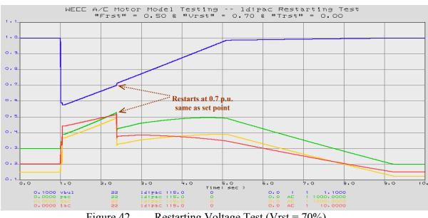
Figure 42. Restarting Voltage Test (Vrst = 70%)
