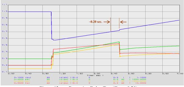
Figure 45. Restarting Delay Test (Trst = 0.20)
