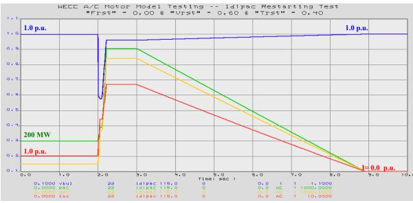
Restarting Fraction Test (Frst = 0%) Figure 37.
