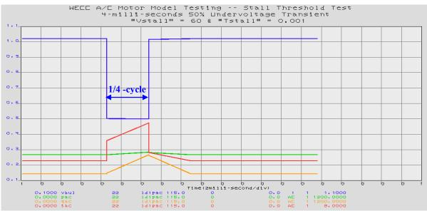
Figure 24. *Stalling Response Time* Test (Vstall=60% - UVsag = 50 % & 4-ms)
