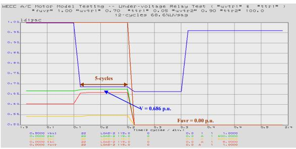
Figure 53. First UV Relay Tripping Parameters Test (*uvtr1*=0.70 & *ttr1*=0.050)
