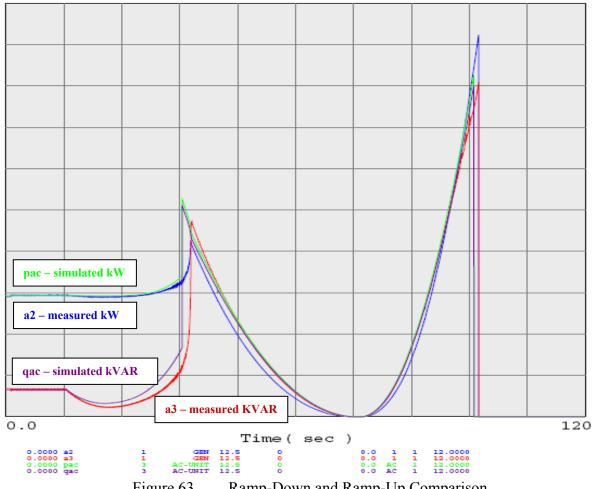
Ramp-Down and Ramp-Up Comparison Figure 63.
