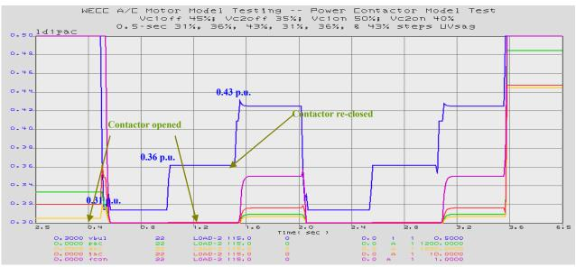
Figure 35. Contactor Second Set of Parameters (Vc2off and Vc2on) Test
