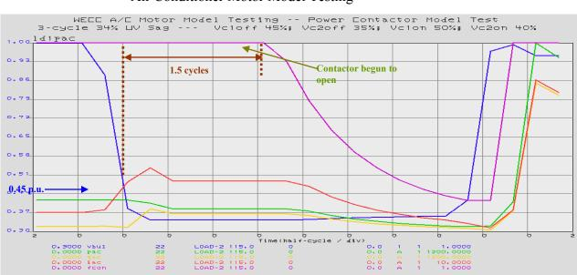
Figure 36. 3-cycles 34 UV Transient Contactor Model Test
