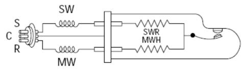
Figure 3. Thermal Overload Protection Switch
