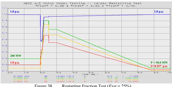
Restarting Fraction Test (Frst = 25%) Figure 38.
