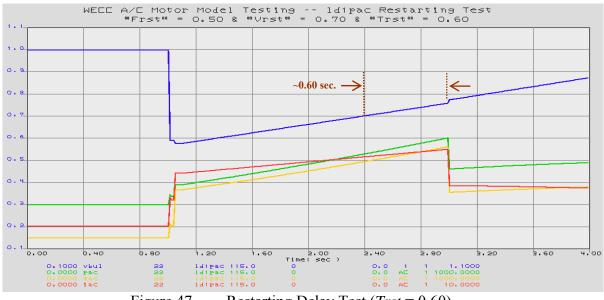
Figure 47. Restarting Delay Test (Trst = 0.60)
