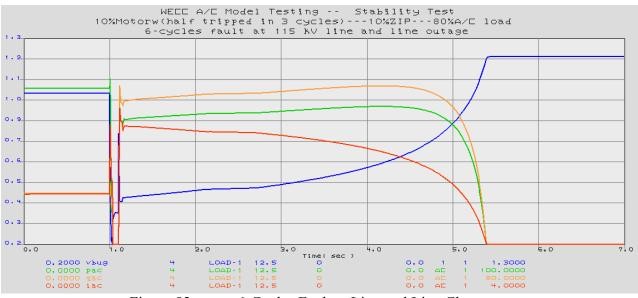
Figure 82. 6-Cycles Fault at Line and Line Clearance
