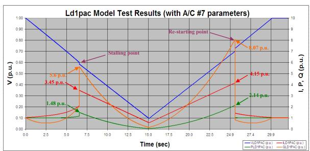
WECC Modeling and Validation Task Force Air Conditioner Motor Model Testing
