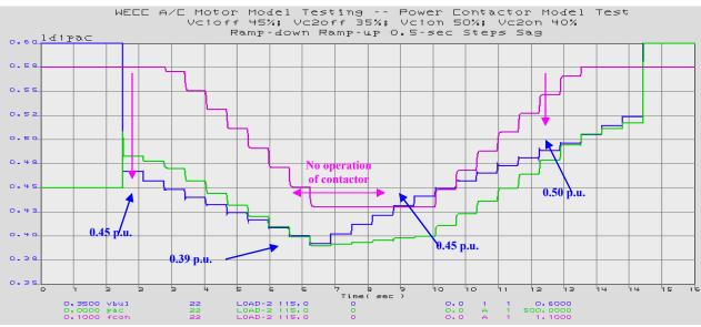
Figure 34. Contactor First Set of Parameters (Vcloff and Vclon) Test
