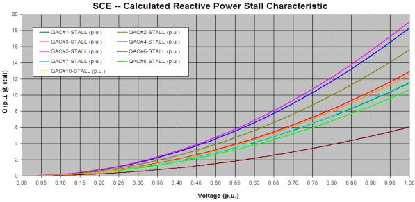
Appendix 2 -- Figure 3. Stall Reactive Power vs. Stall Voltage
