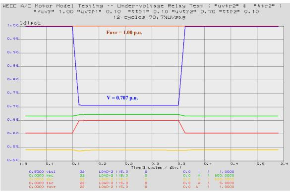
Figure 59. Second UV Relay Tripping Parameters Test (*uvtr*2=0.70 & *ttr*2=0.10)
