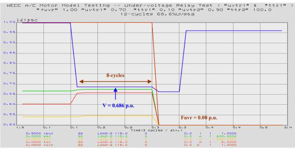
Figure 54. First UV Relay Tripping Parameters Test (*uvtr1*=0.70 & *ttr1*=0.100)
