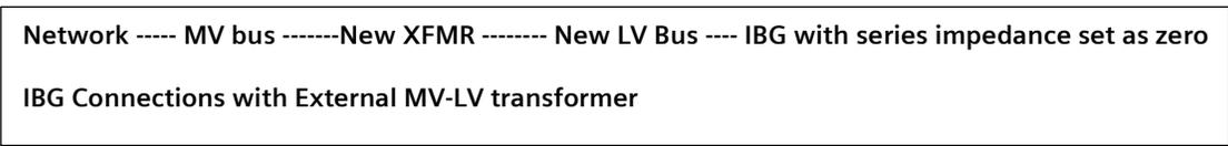
This method allows you to connect more than 1 generator to a common wind-park transformer at the LV bus.
