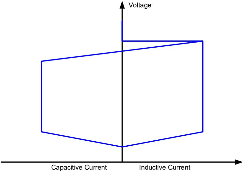
**Figure 2:** VI characteristic of a STATCOM.
