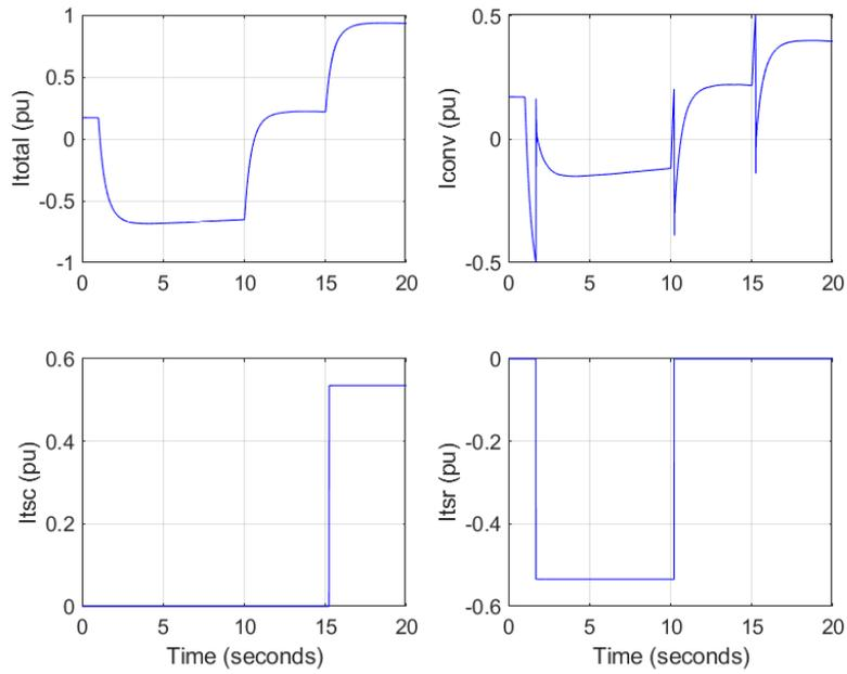
**Figure 7:** Simple example simulation with SVSMO4. A  $V_{ref}$  step was injected to first force the output of the hybrid-STATCOM down at 1 second, and then back up at 10 seconds, and then further up at 15 seconds.
