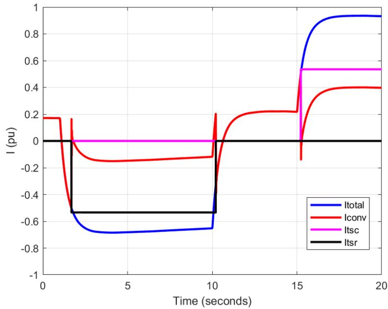
**Figure 8:** Simple example simulation with SVSMO4. A  $V_{ref}$  step was injected to first force the output of the hybrid-STATCOM down at 1 second, and then back up at 10 seconds, and then further up at 15 seconds.
