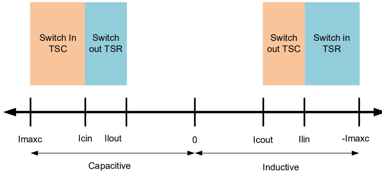
**Figure 6:** Switching logic for the TSC and TSR.
