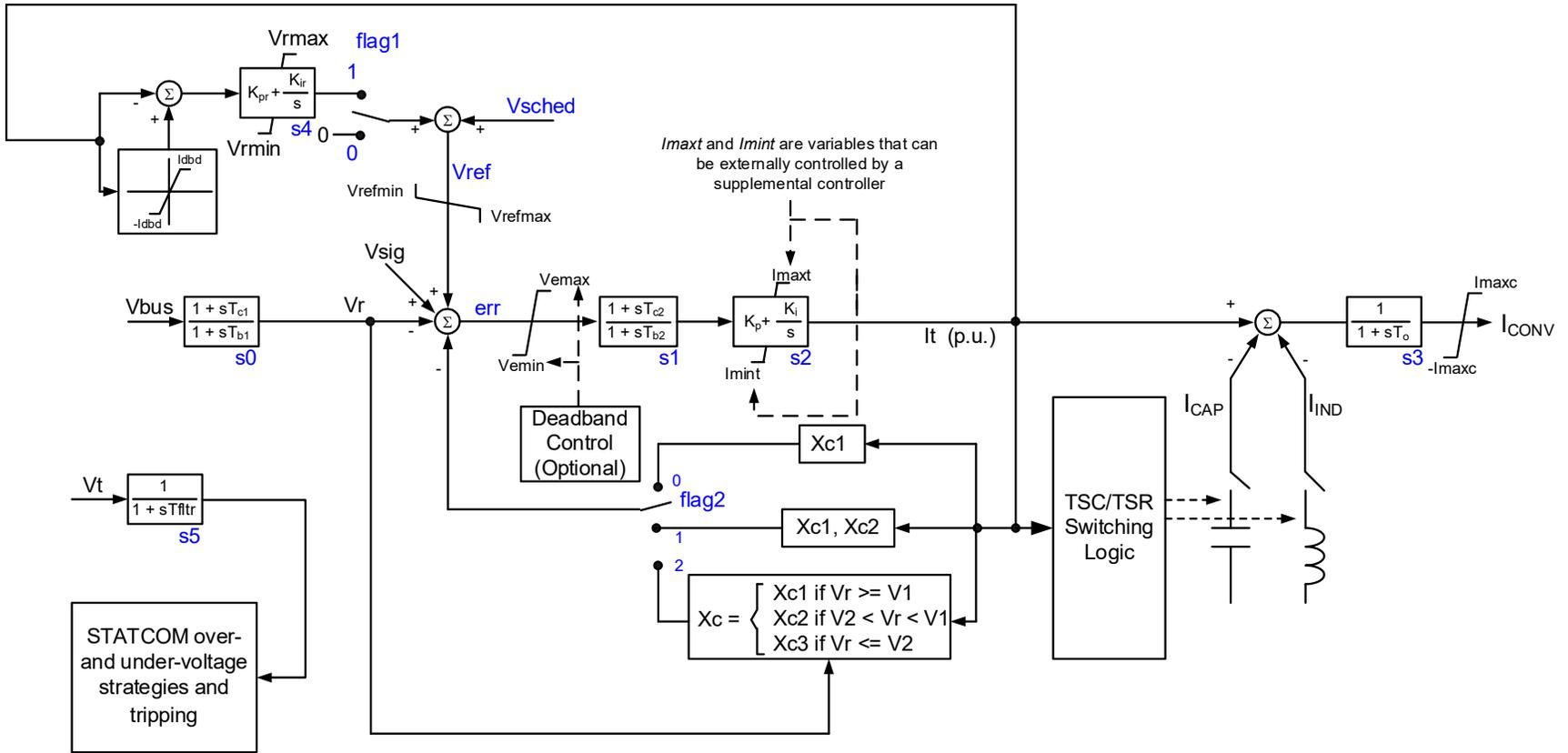
Figure 5: Block diagram of the proposed SVSMO4 hybrid-STATCOM model.
