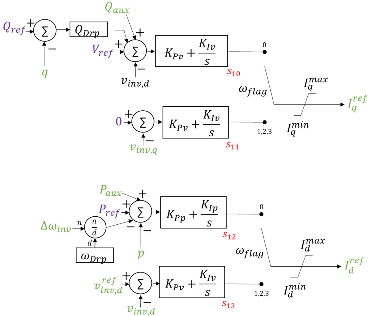
Figure 2: Generic grid forming (GFM) renewable electrical control (REEC\_\*) model
