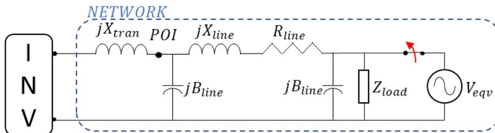
Figure 3: Single inverter-load-equivalent voltage source network to benchmark positive sequence model behavior
