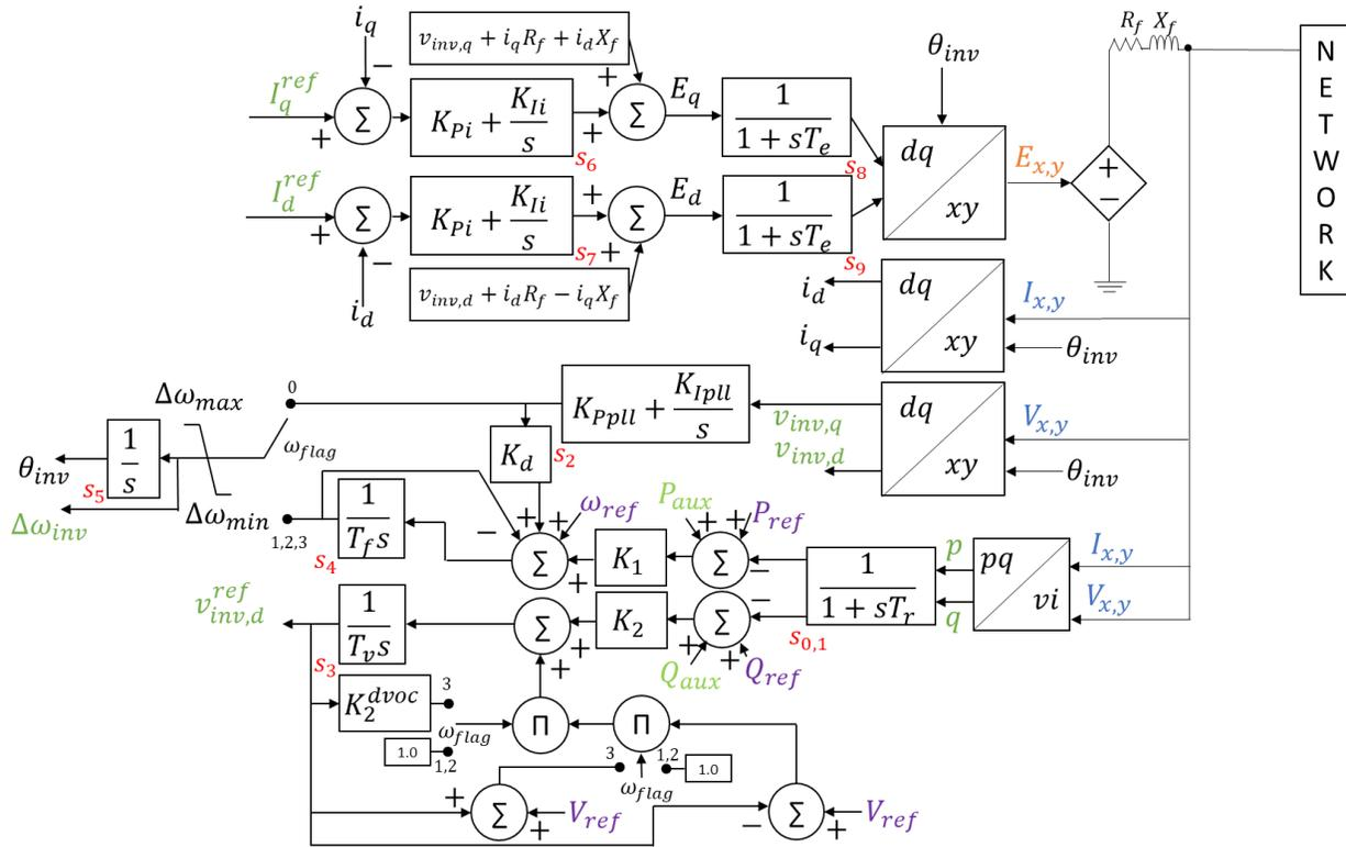
Figure 1: Generic grid forming (GFM) renewable generator/converter (REGC\_\*) model
