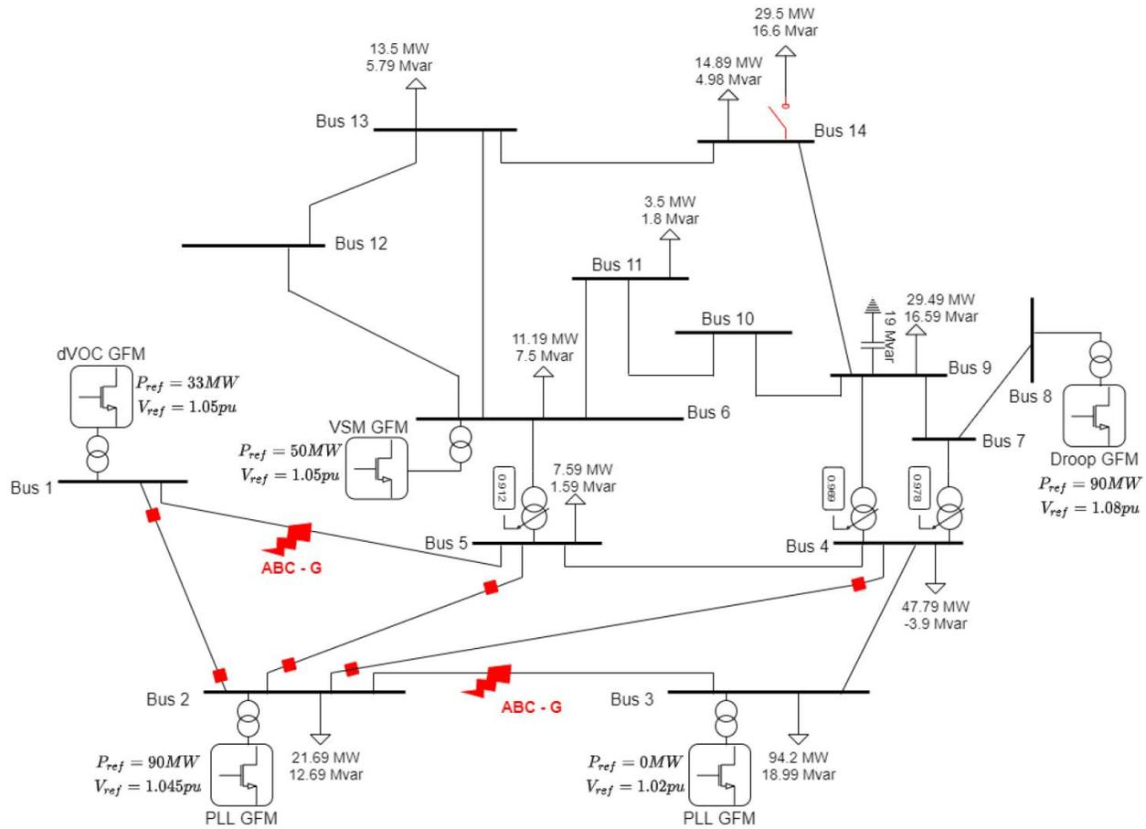
Figure 7: IEEE 14 bus benchmark system topology to benchmark model behavior with multiple IBR sources
