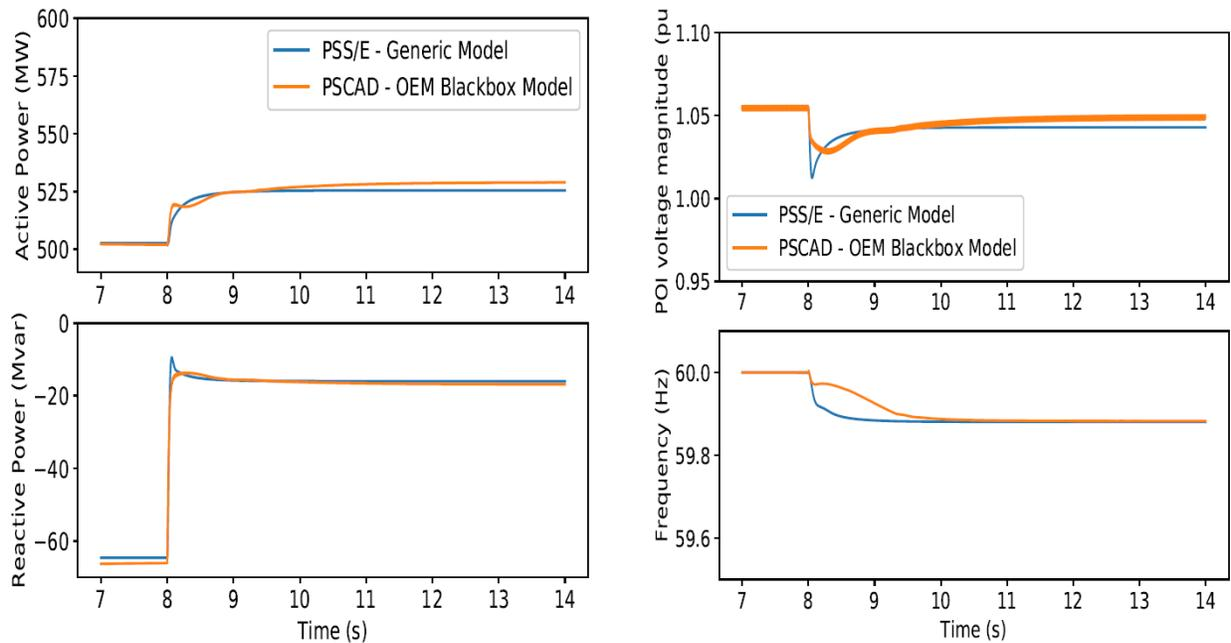
Figure 10: Dynamic response of positive sequence generic model behavior in PLL mode compared against OEM black box EMT model for system islanding event
