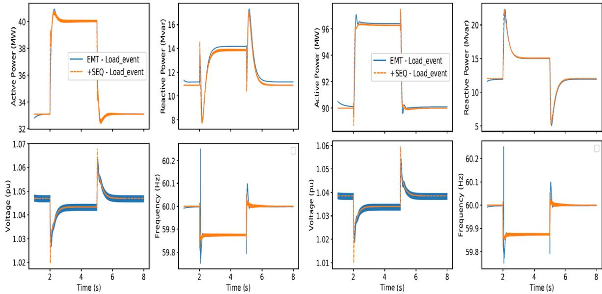
Figure 8: Behavior of IBR at bus 1 (left) and IBR at bus 2 (right) in response to two consecutive load events
