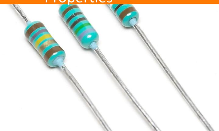
**Resistance (R)** is the property of materials that opposes or resists current by converting electric energy to heat.
